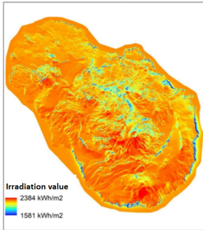
Figure 1.5: Geographical Mapping of Solar Irradiation [12]
