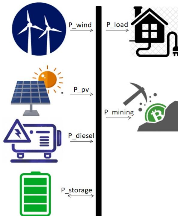
**Figure 3.1:** Simplified network diagram for analyzing power flows and interactions between components in a PyPSA model of an electrical system with Bitcoin mining and storage units
