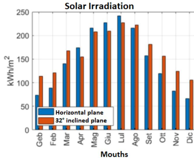
Figure 1.4: Visualization of Monthly Solar Irradiation Throughout the Year [12]
