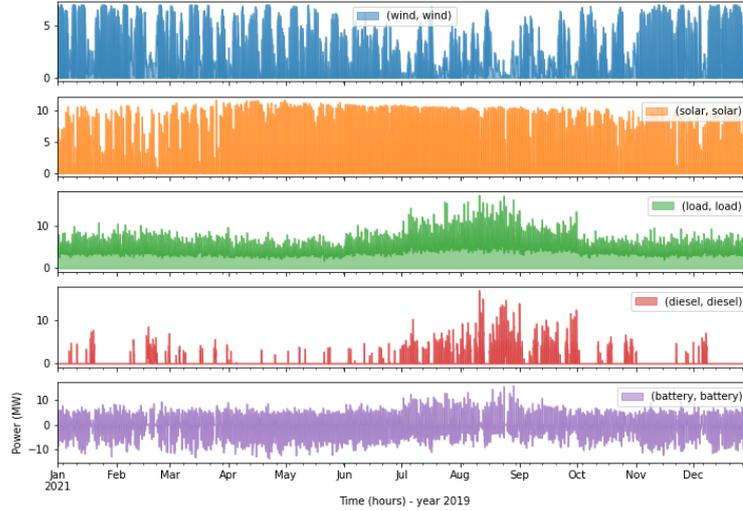
**Figure 5.2:** Scenario 1: Key Components of the Network Representation
