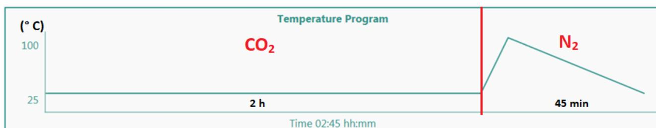
Figure 17 – TGA process for CDs in natural state.
