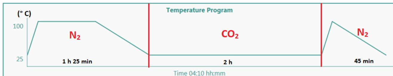
**Figure 24** – Schematic TGA process of CDs with an initial dehydration step.
