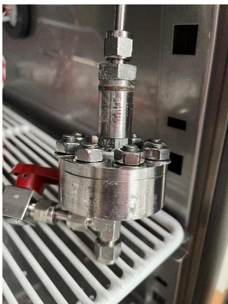
*Figure 30: housing in a climate chamber, with feed in higher side and permeate in the lower side.*
