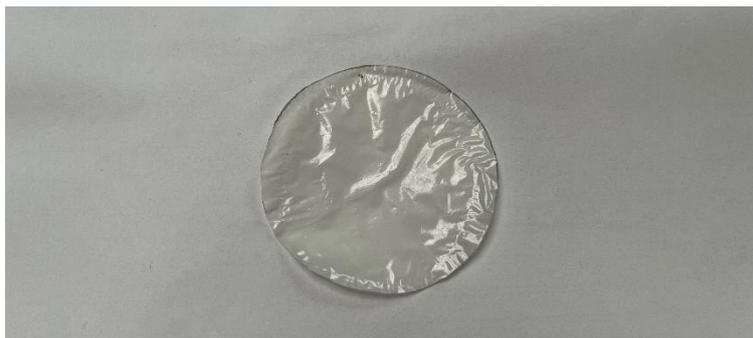
Figure 23: PES-WC membrane made by chemical department of UNITO and tested in our bench.
