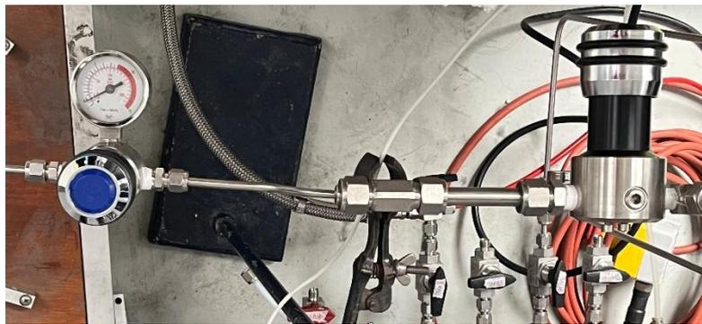
Figure 29: two pressure reducers in series able to stabilize feed pressure during tests.
