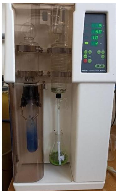
Figura 3.6: BUCHI Distillatore Kjeldahl UNI B-323
