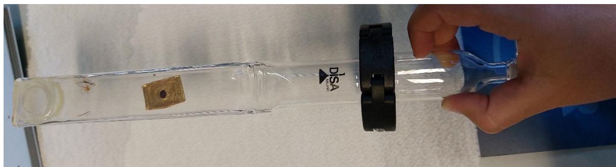
Figure 3.9 Handmade quartz cell with KBr window used for FT-IR measurements, containing the self-supporting pellet.
