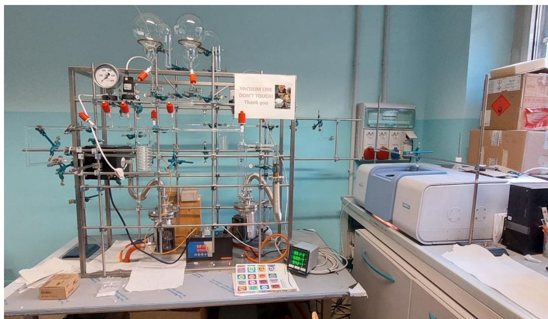
Figure 3.8 FT-IR setup for analysis. On the right: BRUKEREQUINOX-66 spectrometer. On the left: vacuum line
