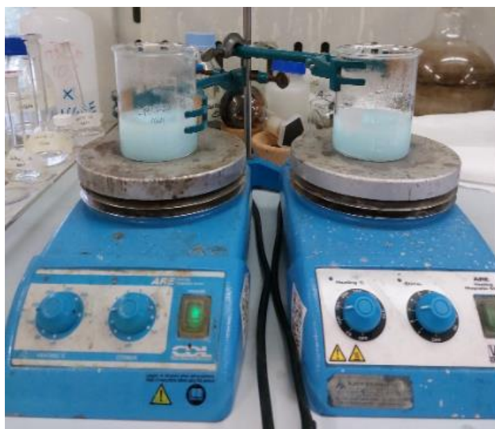
Figure 3.3 Synthesis of impregnated samples. A hot plate stirrer enables both the mixing and the heating of the solution, until complete evaporation of the water.
