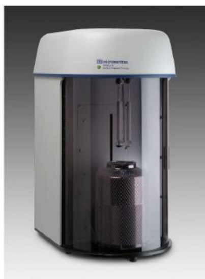
Figure 3.10 Picture of Tristar II 3020 Micromeritics, the equipment employed for the physisorption.
