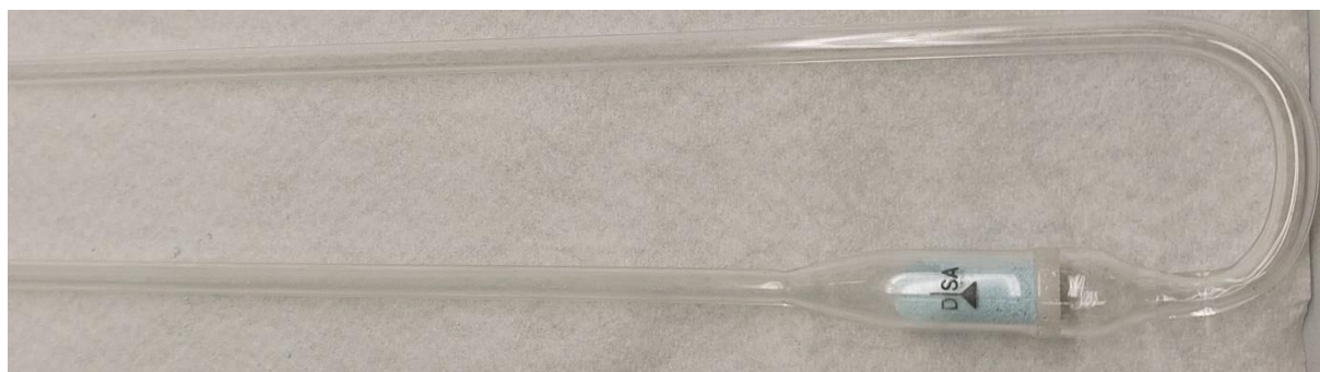
Figure 3.5 Tubular quartz reactor for calcination
