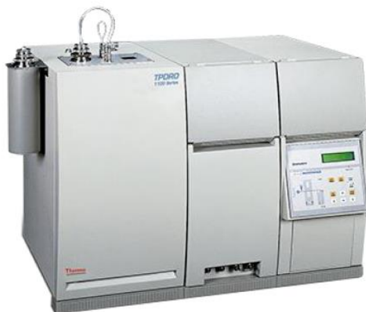
Figure 3.7 Thermoquest CE instruments TPDRO 1100 employed for the H 2 -TPR analysis
