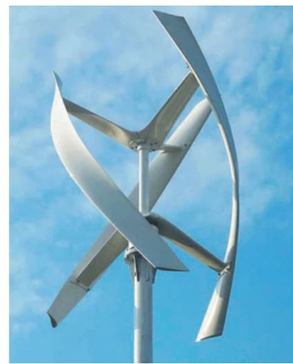
Fig.51: UGE's innovation is the helical blade design, which adds aesthetic appeal.
