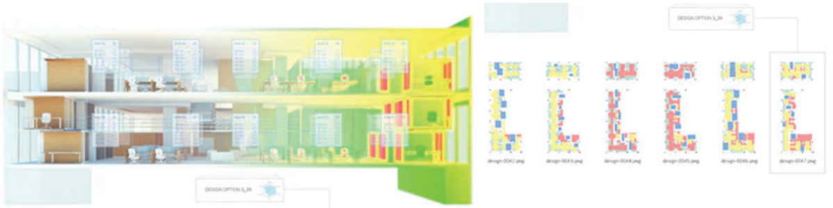
Fig.17: MaRS generative project, It involves the integration of a rule-based geometric system, a series of measurable goals, and a system for automatically generating, evaluating, and evolving large number of design options. (Autodesk).
