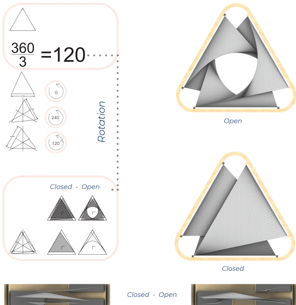
Fig.55: Trinary case (Trinary unit) structure logic and components - plans and sections.
