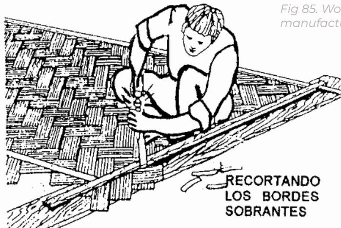
Fig 85. Woven panel manufacturing process
