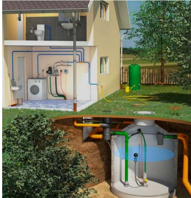
aerated. Filtration removes large particulate matter, which frequently both carries and feeds bacteria. Removal of this particulate matter, along with oxygenation of the water, greatly reduces the amount of harmful bacteria in the tank.
