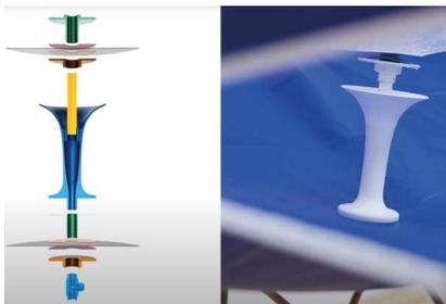
Figure 54: Water collection system(funnel)
