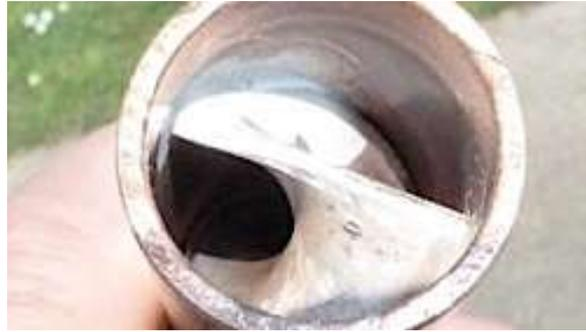
Figure 45: Section of the pipe (double spiral inside Vortex Water Revitalisers)
