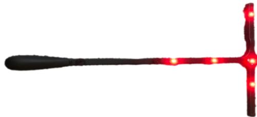
**Figure 7.2:** Active Wand for the optical stereo-photogrammetric system calibration
