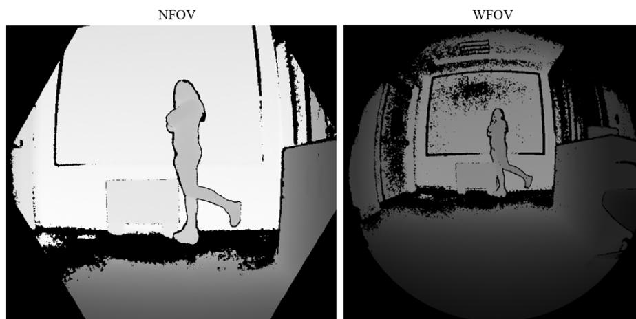
**Figure 5.2:** Examples of depth images taken with narrow field-of-view (left) and wide field-of-view (right) mode.
