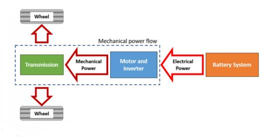
Fig. 1.1: Electric vehicle power flow [2]
