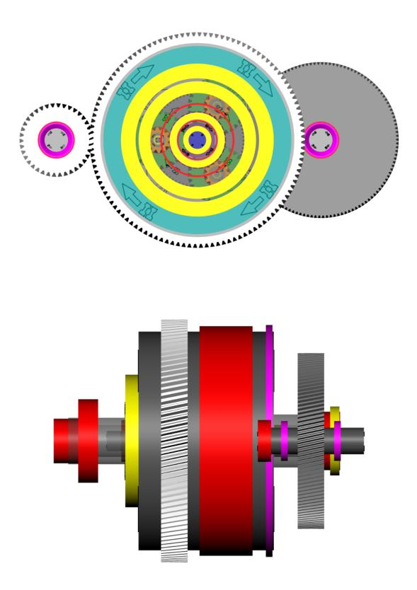
Fig. 4.12: Frontal and left views of the two-speed model in KISSsys
