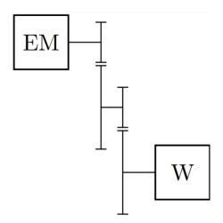
Fig. 3.1: Stick diagram of a one-speed transmission [30]
