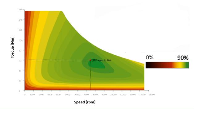
Fig. 4.14: Motor efficiency map with the operating point for  $i_{2,def}$  [34]
