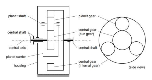
Fig. 4.2: Example of a single PGT [32]
