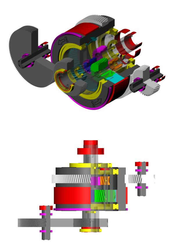
Fig. 4.13: Front/left and top cut views of the two-speed model in KISSsys
