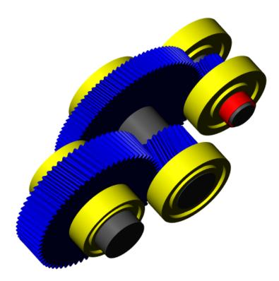
Fig. 3.6: KISSsys diagram of the one-speed transmission
