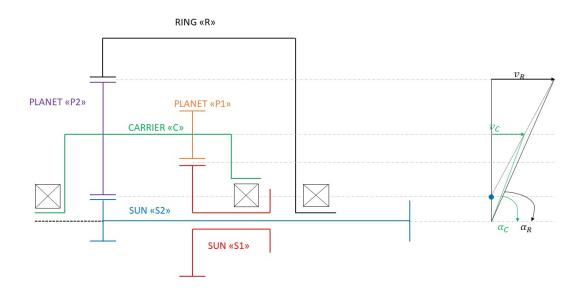
Fig. 4.5: Stick diagrams of the first gear ratio  $i_{CR,1}$  and the second gear ratio  $i_{CR,2}$
