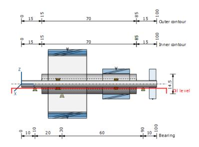
Fig. 4.8: Sketch of the stepped planet shaft for the two-speed transmission
