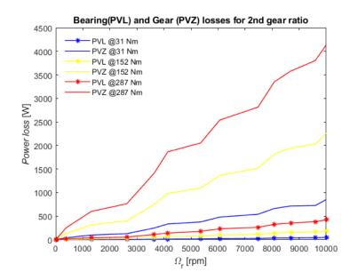
Fig. 5.7: Bearing losses of the two-speed transmission for the second gear ratio
