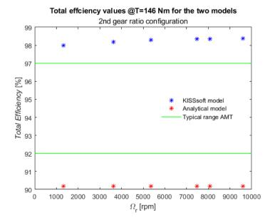
Fig. 5.6: Comparison of few total efficiency values in the second gear configuration
