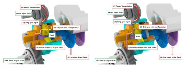
Fig. 4.4: Working condition for the first and second gear ratio realization, respectively [33]
