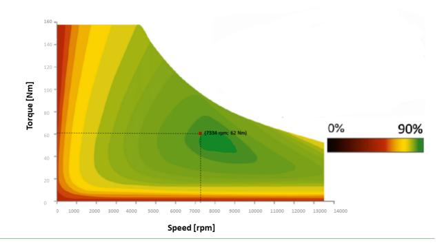
Fig. 4.6: Motor efficiency map with the operating point for  $i_{2,ref}$  [34]
