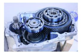
Fig. 2.5: Single speed gearbox of Tesla Roadster's prototype 1.5 powertrain [23]
