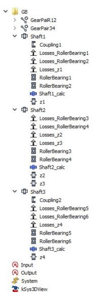
Fig. 3.4: KISSsys model tree of the one-speed transmission
