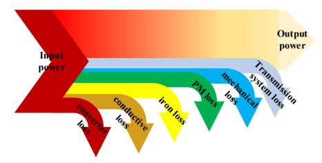
Fig. 2.7: The various loss components of the propulsion system of EVs [26]
