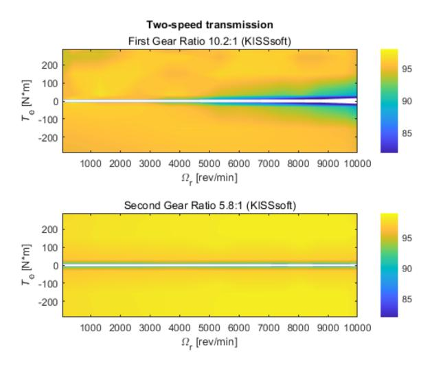
Fig. 5.3: Efficiency maps of the two-speed model in KISSsoft
