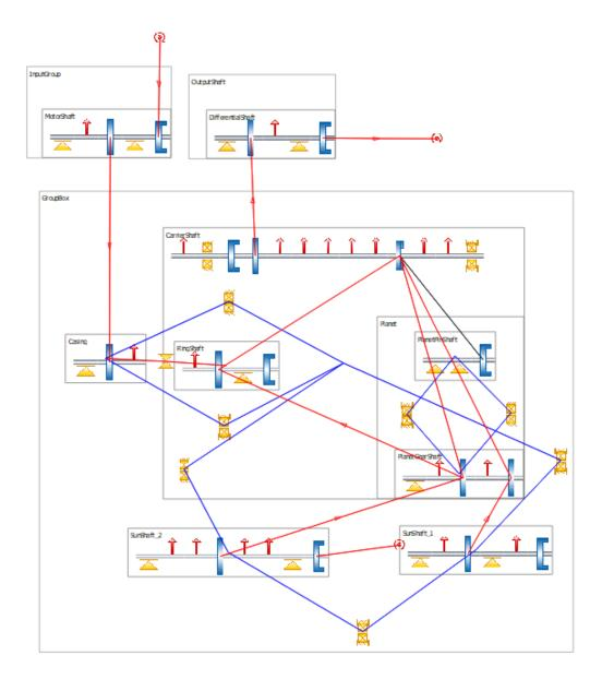
Fig. 4.11: KISSsys diagram of the two-speed transmission
