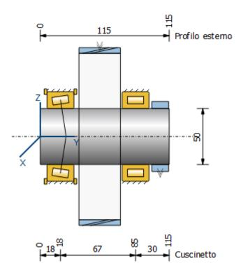
Fig. 3.9: Sketch of the output shaft for the one-speed transmission
