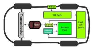
Fig. 1.7: Configuration of a parallel FCHEV [3]
