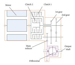
Fig. 2.6: Representation of DCT for the EV powertrain [24]
