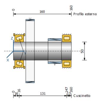
$\label{eq:Fig. 3.8: Sketch of the countershaft for the one-speed transmission$
