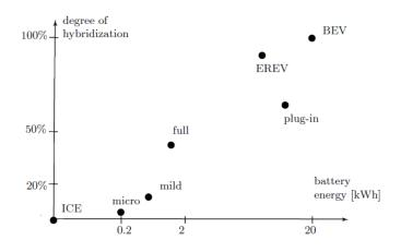
Fig. 1.5: Degree of hybridization for HEV [1]
