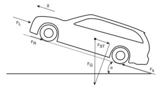
Fig. 2.1: Forces on a vehicle driving at constant velocity [16]
