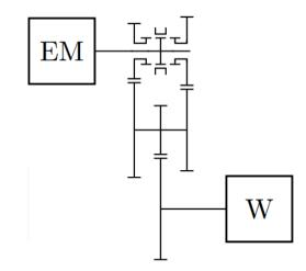
Fig. 4.1: Stick diagram of a two-speed ATM transmission [30]
