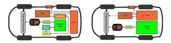
Fig. 1.4: Configuration of a series HEV (left) and a parallel HEV (right) [3]
