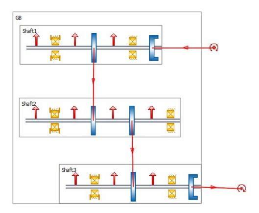
Fig. 3.5: KISSsys diagram of the one-speed transmission
