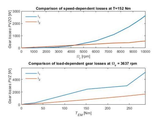
Fig. 5.4: Comparison of the speed- and load-dependent gear loss for the two gear ratios
