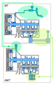
Fig. 2.3: Conversion of the MT in AMT: in blue the replacement of the clutch pedal with an electrohydraulic / electrical actuator, in green the substitution of the shift lever with an electronic controlled gear actuation mechanism [17]
