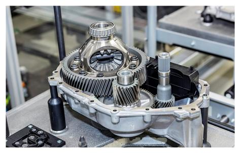
Fig. 3.2: Gearbox of VW ID.3 Pro Performance [31]
