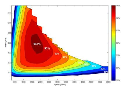
Fig. 1.9: Permanently Excited Synchronous motor (PMSM) efficiency map, source: x-engineer.org
