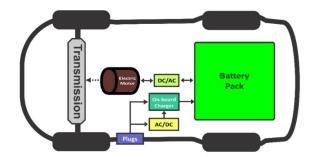
Fig. 1.3: Configuration of a BEV [3]
