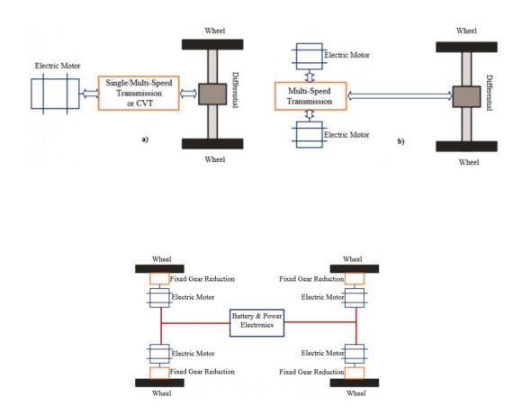
Fig. 1.12: Centralised (top) and distributed (bottom) drive systems [4]
