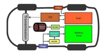
Fig. 1.6: Configuration of a parallel PHEV [3]
