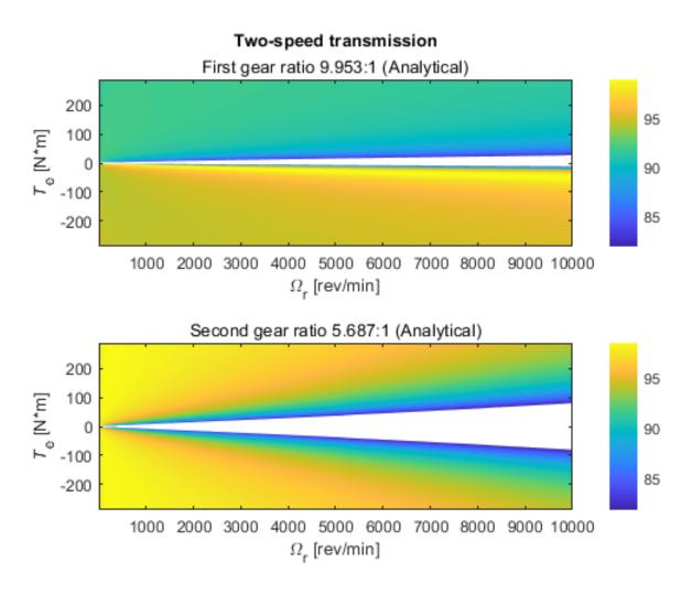
Fig. 5.5: Efficiency maps of the two-speed model with the analytical approach
