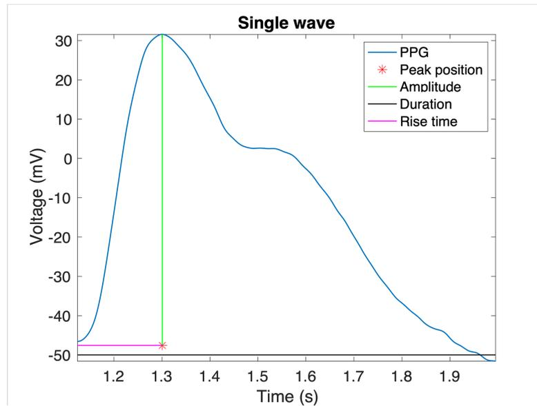
**Figure 5.5:** An example of a PPG wave.
