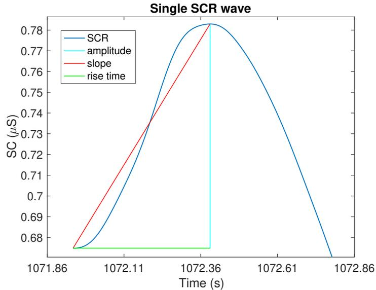
**Figure 5.3:** Example of a single SCR wave.
