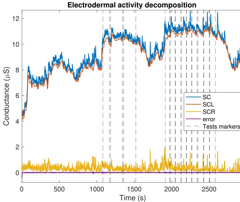
**Figure 5.2:** [41] Decomposition of EDA signal in SCL, SCR and error, obtained through the CVX method proposed by Greco et al.
