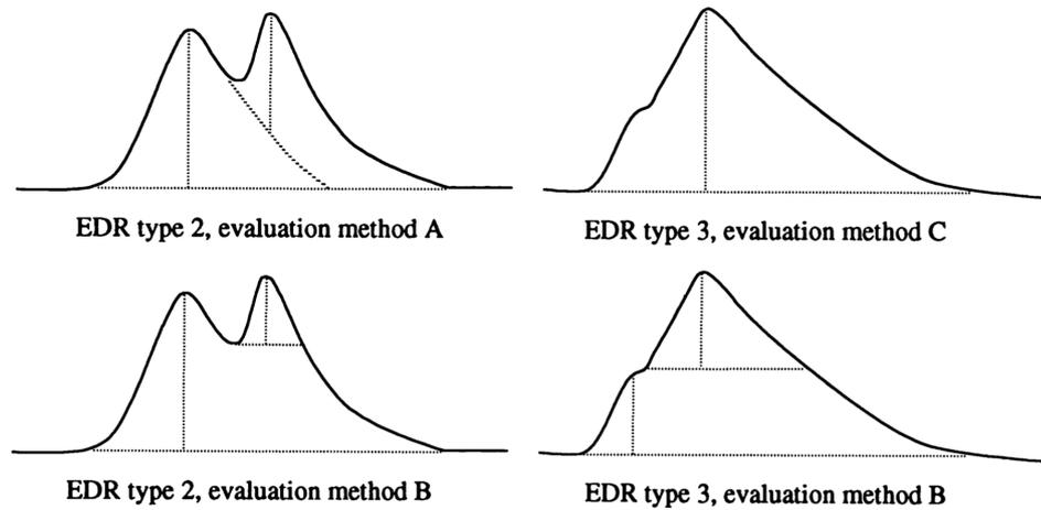
**Figure 3.4:** [3] Four examples of overlapping SCR. It is possible to distinguish two other different types of waves, distinguishable (2) and non-distinguishable(3) evaluated with three criteria: (A) measures the amplitude of the second peak from the interpolated recovery line of the first; (B) is the *standard* method which evaluates the amplitude with respect to the second wave start; (C) in this case the first peak is not considered.
