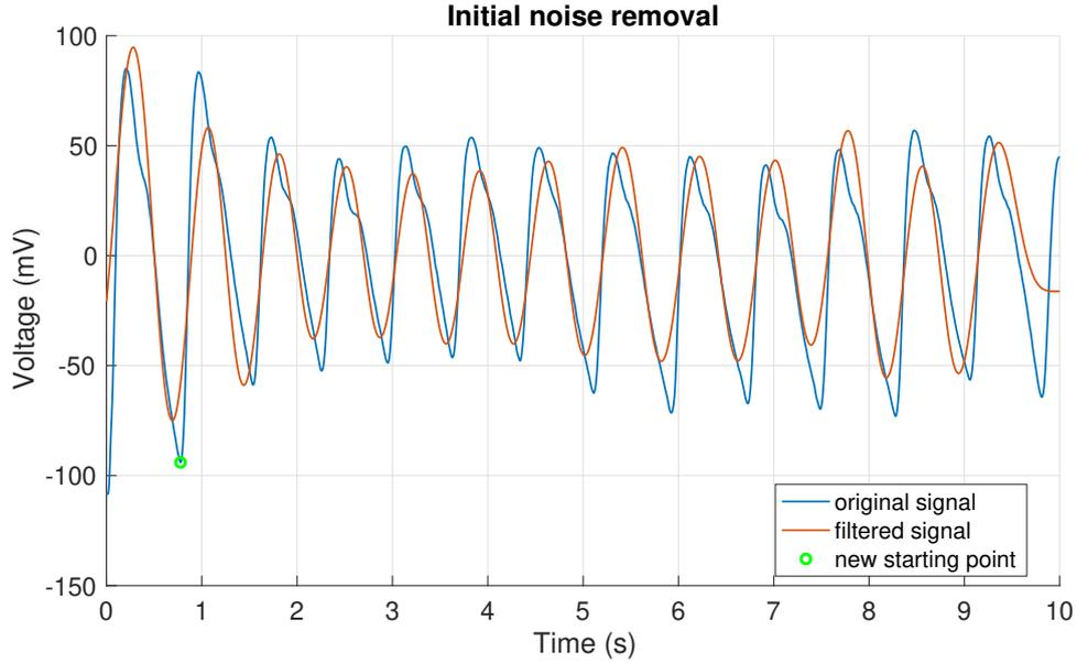
**Figure 5.1:** Signals new starting point selection from a few second window of the beginning of PPG.
