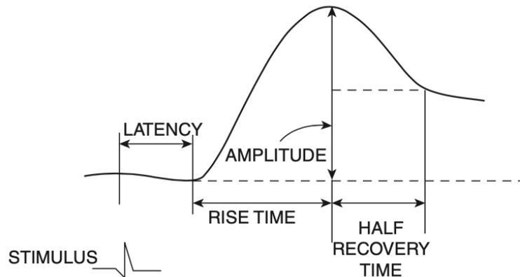
**Figure 3.3:** [25] Graphical representation of principal SCR components in a typical wave (Type 1[3]).
