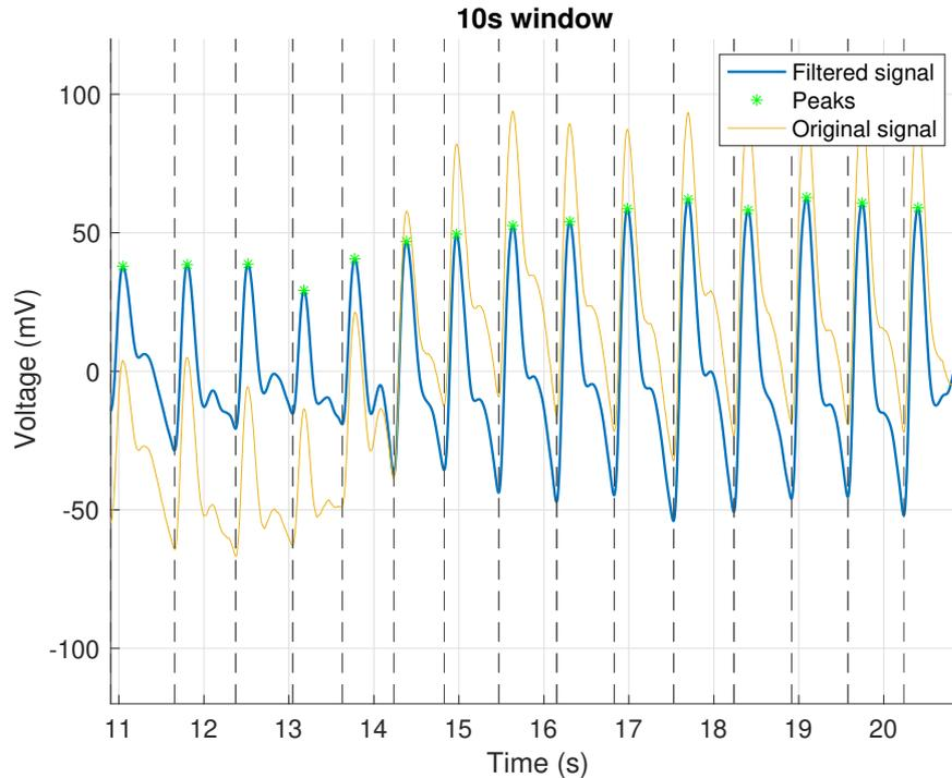
**Figure 5.4:** 10s window of PPG signal.
