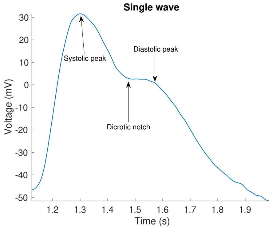
**Figure 3.5:** Graphical representation a typical PPG wave from one of the subjects' signals.
