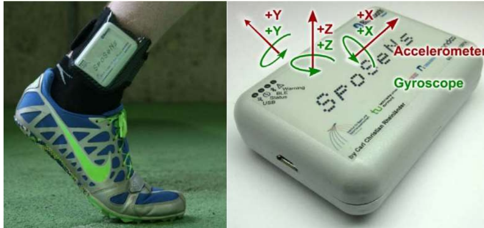
Figure 2-5 In the figure, taken from [62] , the IMU device used in this paper and its positioning on one of the athletes is shown.
