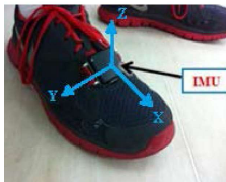
Figure 2-9- In the figure, taken from [68], the positioning of the IMU is shown.
