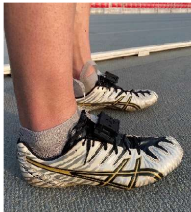
Figure 2-3 – Subject equipped with MIMUs affixed to the shoelaces of each shoe and with sensorised insoles.
