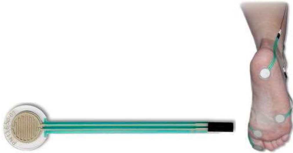
Figure 1-12 – example of foot switch and their positioning. Source: https://www.motion-labs.com/prod_access_footswitches.html
