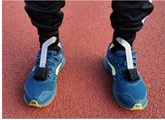
Figure 2-1 – Subject wearing the INDIP multisensory sistem and sensorised insoles.
