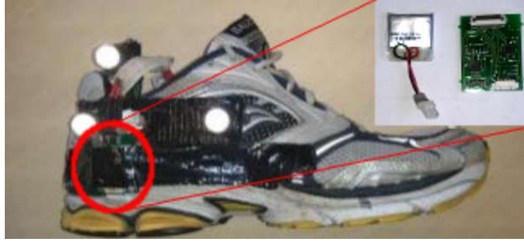
Figure 2-7- In the figure, taken from [64], the IMU and its placement on the shoe is shown.
