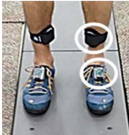
Figure 2-8- Figure taken from [67] that shows the positioning of four of the IMUs used in their study.
