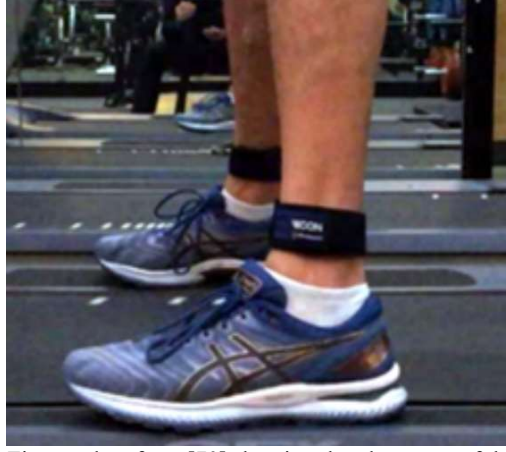
Figure 2-10- Figure taken from [70] showing the placement of the IMU on the ankle
