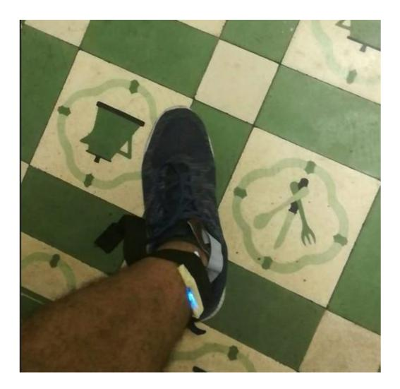
The user was wearing the insole inside the shoe and the IMU was mounted on the ankle as shown in the previous picture. You should consider that in this case the angles of the gyroscope roll and yaw will be inverted.
