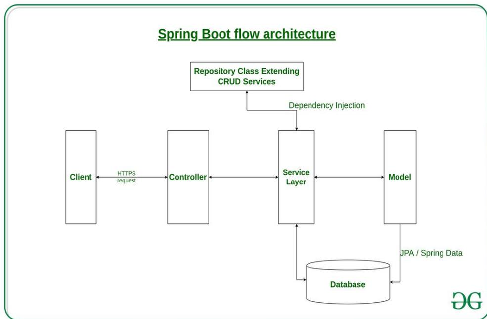
Figure 3.2: Spring boot architecture [15].
