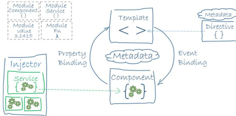
Figure 3.1: Angular applications' structure [12].
