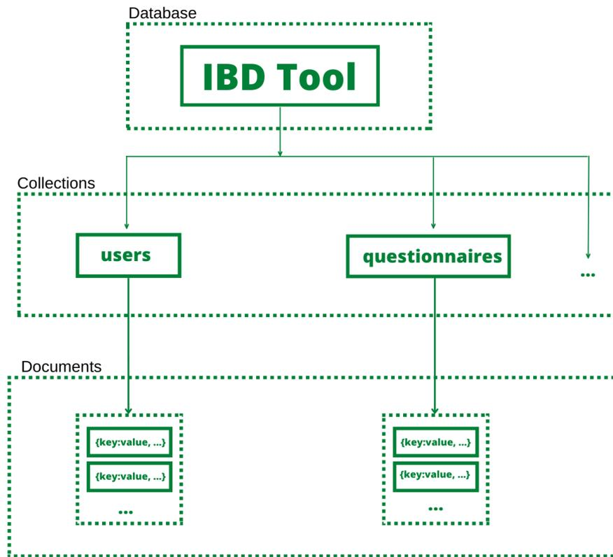
**Figure 3.4:** IBD Tool database structure.
