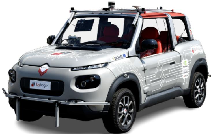
**Figure 6.1:** VeGA, autonomous vehicle
