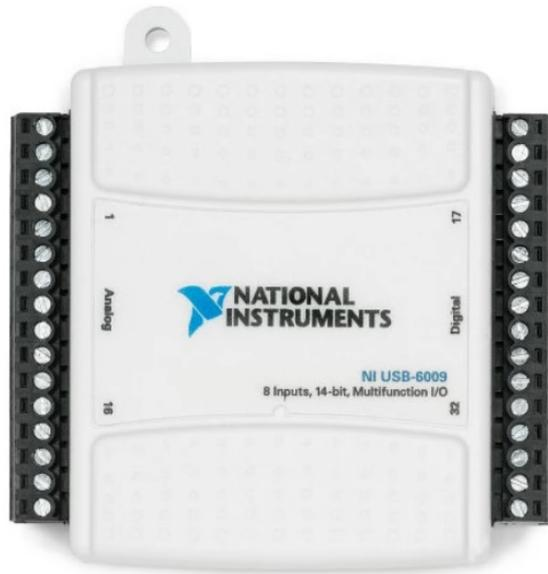
**Figure 2.4:** USB-6009 acquisition device
