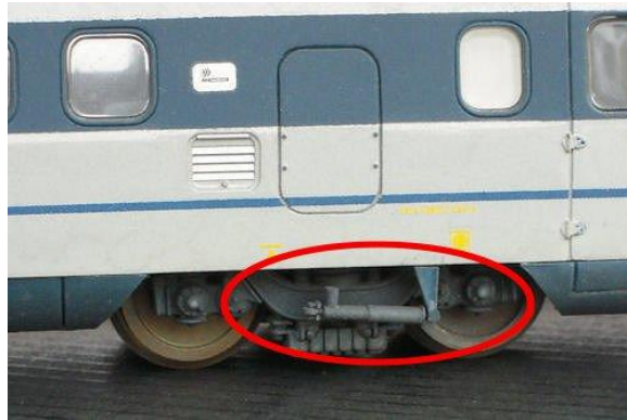
Figure 2.1 Damping between carriage and fixed point of the body
