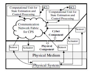
Figure 2.1. View of a Cyber-Physical System [4]
