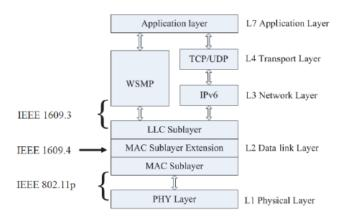
Figure 2.4. Protocols used in ISO/OSI stack [11].
