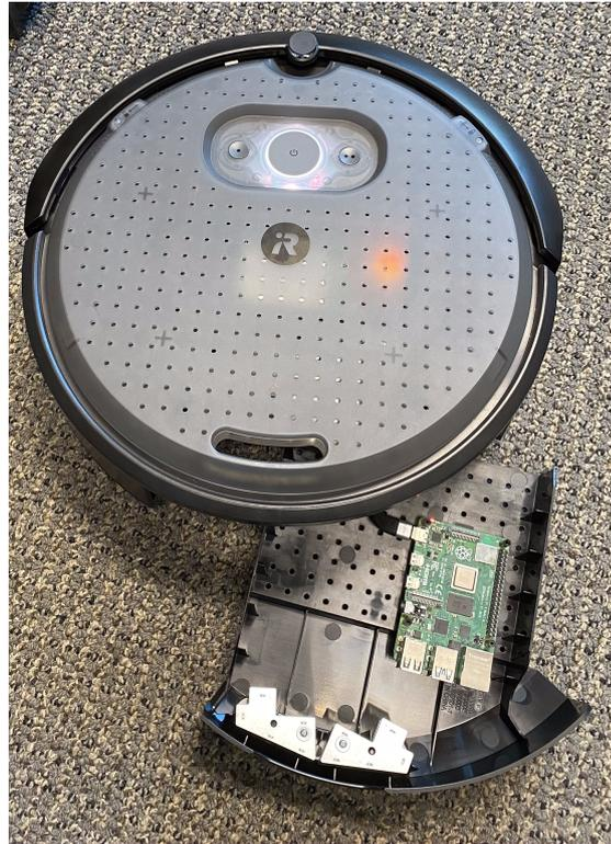
**Figure 3.6:** Raspberry Pi 4 installation on Create 3.
