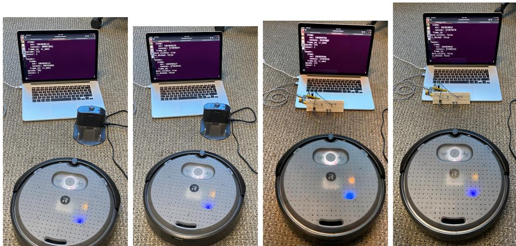
Figure 2.7: Comparison between the actual dock opcodes and the dock replica mounting three LEDs.
