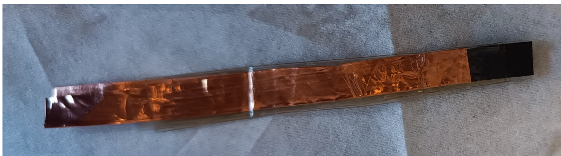
Figure 2.16: GDE electrodes tested with CV measurements
