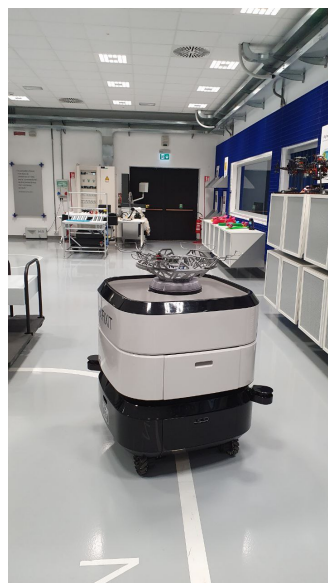
(c) Arrived at the end of the hallway, the AMR decides to move towards the centre of the laboratory, to acquire more information about the environment
