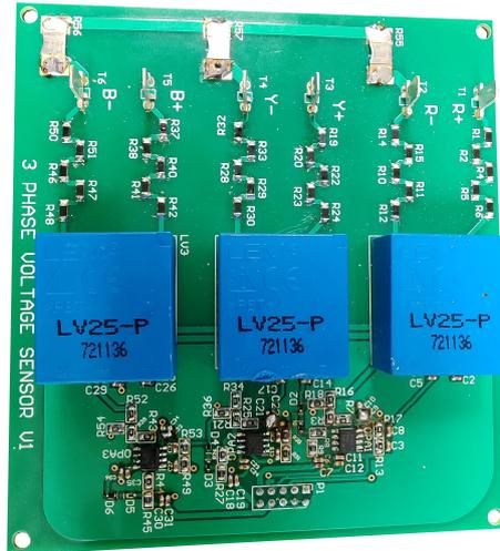
Figure 3.25: DC voltage sensor board
