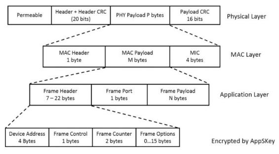
Figure 3.11: LoRaWAN frame format[36].
