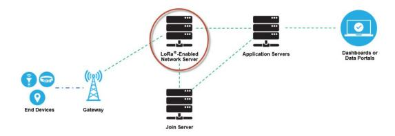
Figure 3.9: LoRaWAN Network Server in a LoRaWAN network deployment[29].
