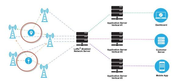
Figure 3.8: Gateways receiving and transmitting messages from end devices[29].
