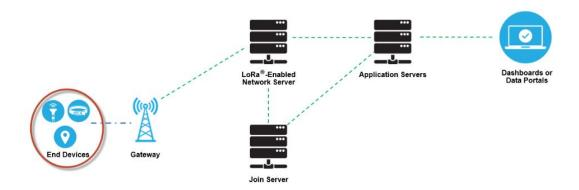
Figure 3.7: End devices in LoRaWAN network deployment[29].
