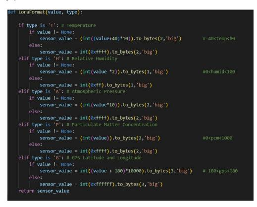
Figure 5.17: Update LoRa buffer function.
