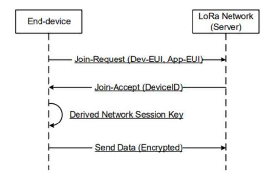
Figure 3.3: Overview of the OTAA Join procedure[23].
