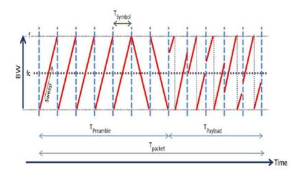
Figure 5.13: Chirps containing preamble and payload [57].
