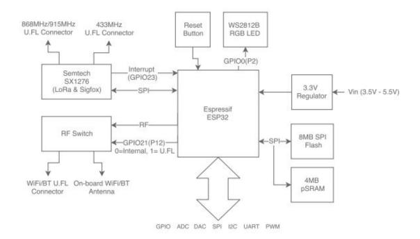
Figure 4.4: Block Diagram of LoPy4.[45]
