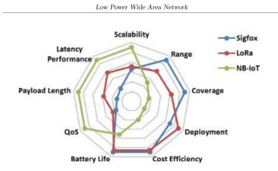
**Figure 2.1:** Respective advantages of Sigfox, LoRa, and NB-IoT in terms of IoT factors[4].
