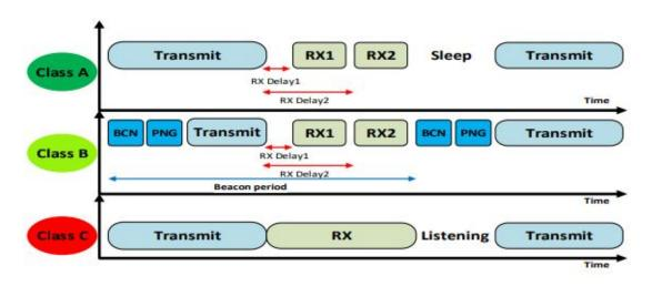
Figure 3.10: Class time diagram of LoRaWAN devices [34].
