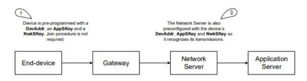
Figure 3.4: ABP End Device Activation[23].
