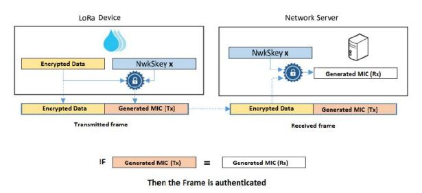
Figure 3.13: Frame authentication by the Network Server[42].
