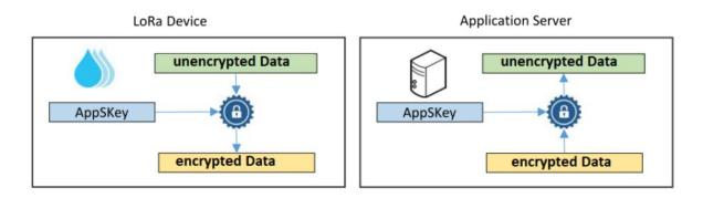
Figure 3.14: Data encryption/decryption.[42]
