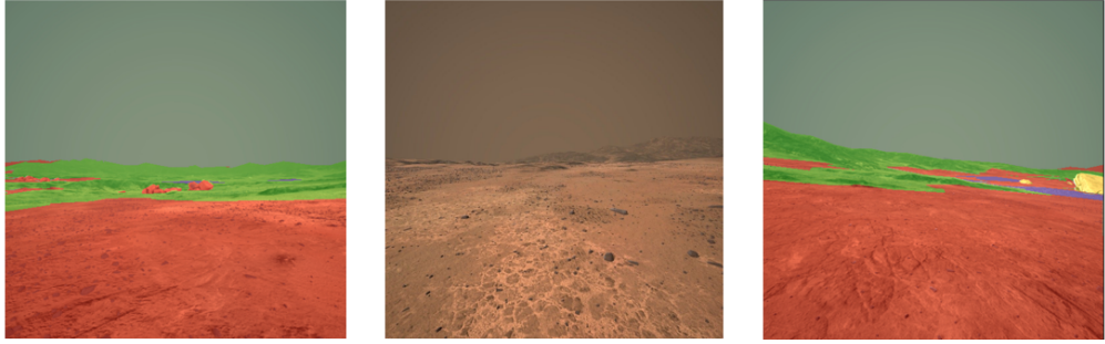
Figure 4.4: Example from synthetic rover dataset: Red: Soil, Green: Bed Rock, Blue: Sand, Yellow: Big Rock. Picture in the middle represents original image without label
