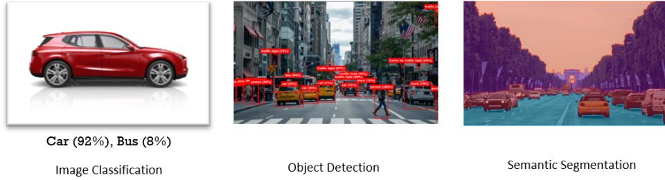
Figure 1.2: Differences between some of the tasks from computer vision
