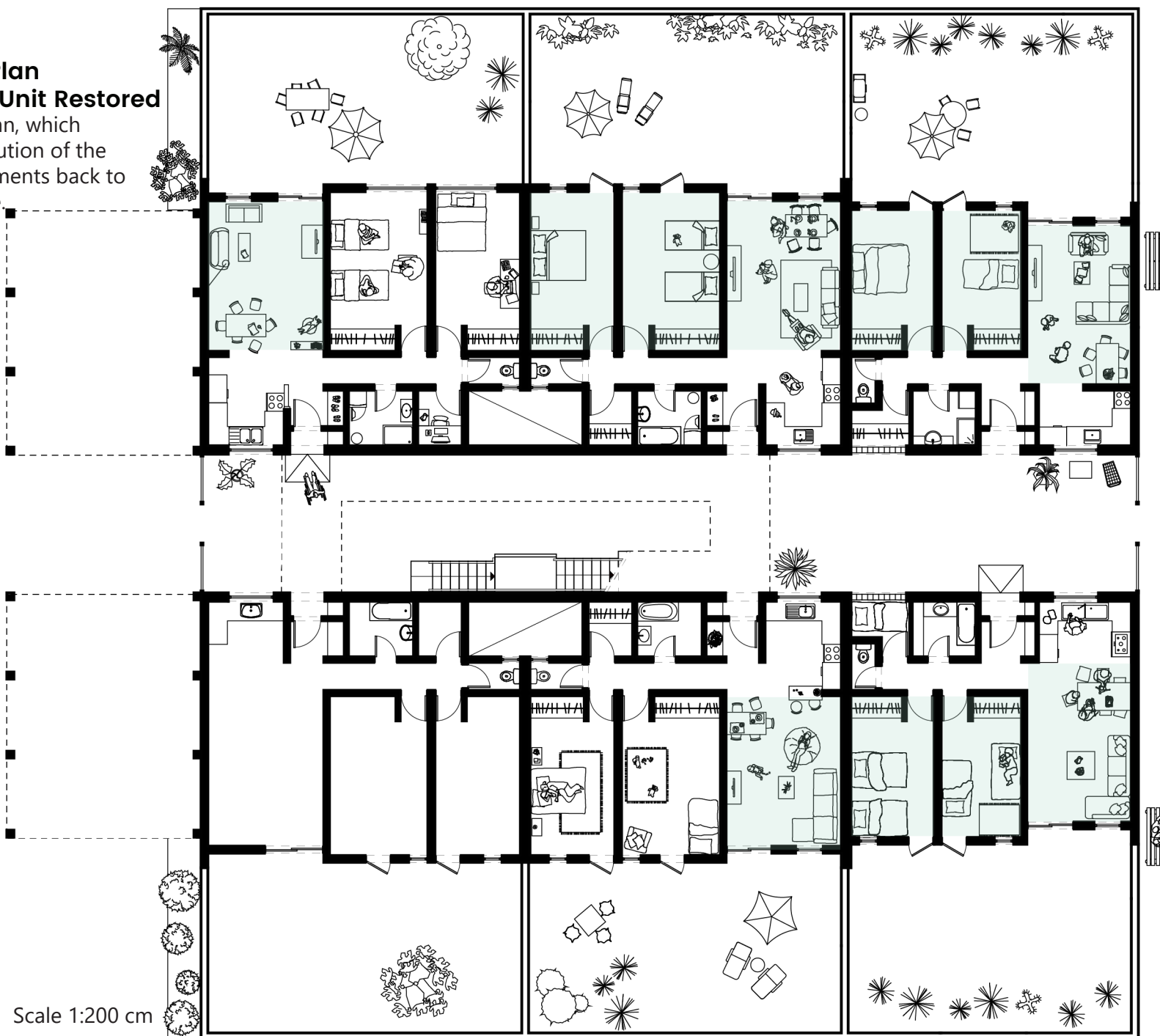
Fig 114. Restoration of Patio residential unit, Ground Floor plan of the project, spaces restored to a regulated conditions are highlighted in green. scale 1:200. Source: elaborated by the author.
