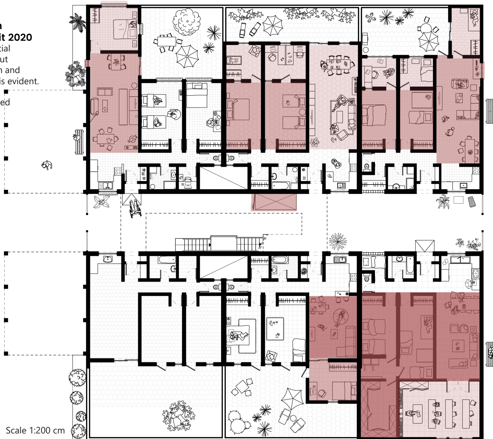
Fig 113. Problematic spaces in the ground floor plan of the patio unit, lack of natural lighting, ventilation and air exchange, are highlighted in red. scale 1:200. Source: Elaborated by the author.
