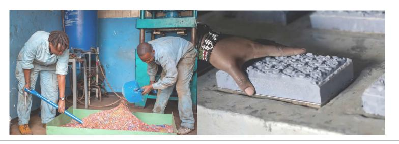
Gjenge Makers use plastics waste shredded into small pieces and mix it with sand. The mix is then transferred into an extruder (heating machine). At 367°C, the materials are heated and mixed further, slowly turning into a gelatinous blob.
