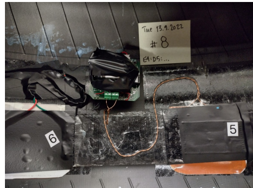
(b) Position of the tribo harvester in the tire from Nokian Tyres
