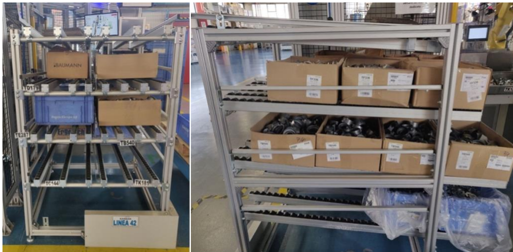
Figure 68: Front and Side View Gravity Flow Rack L42
