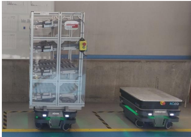
Figure 24: MiR 250 with Fixed Gravity Flow Rack & MiR 250 Shelf Carrier Module
