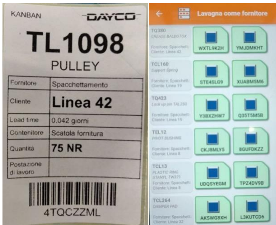
Figure 23: Kaban Label L42(on the left) and KanbanBOX software (on the right)
