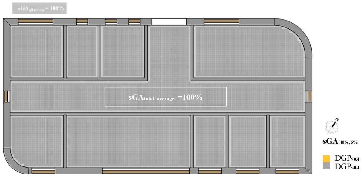
*Figure 4.45 Spatial Glare Autonomy (sGA) heatmap for the multi-zone model, louver shades*
