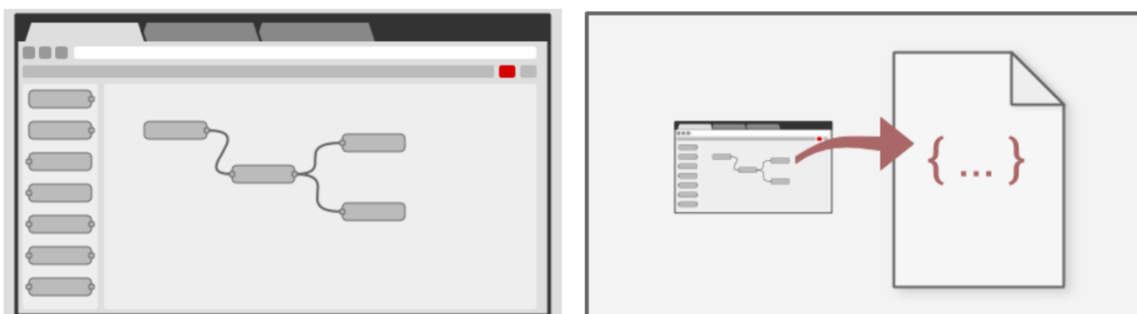
Figure 2- 8 On the left the creation of a flow with four nodes; on the right the programming environment available for each node
