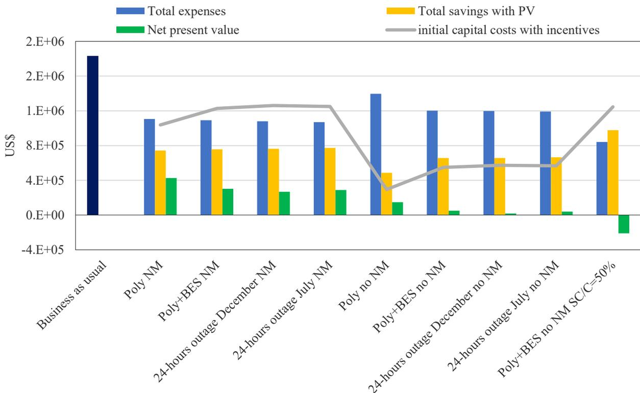
Figure 91. Total energy expenses, total energy savings with PV, net present value and initial capital costs after incentives using polycrystalline for the detached block. Poly = polycrystalline, NM = net metering, BES = battery energy storage.
