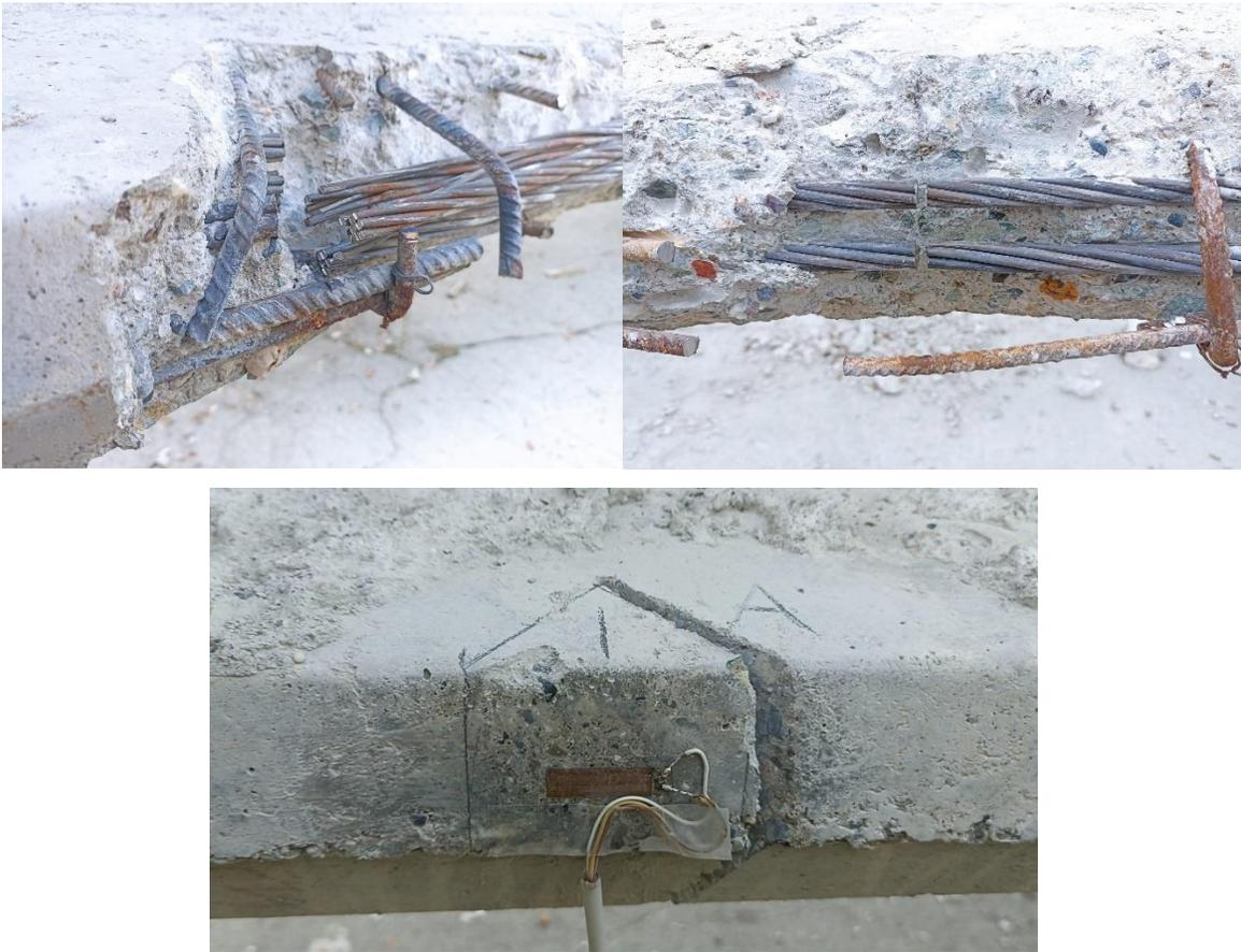
*Figure 3. (a & b) Strand cuts. (c) Concrete relax (saw-cuts) test.*
