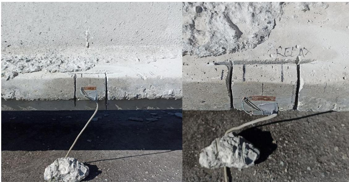
*Figure 25. Concrete relax test on beam 1, point A (left), and point B (right).*
