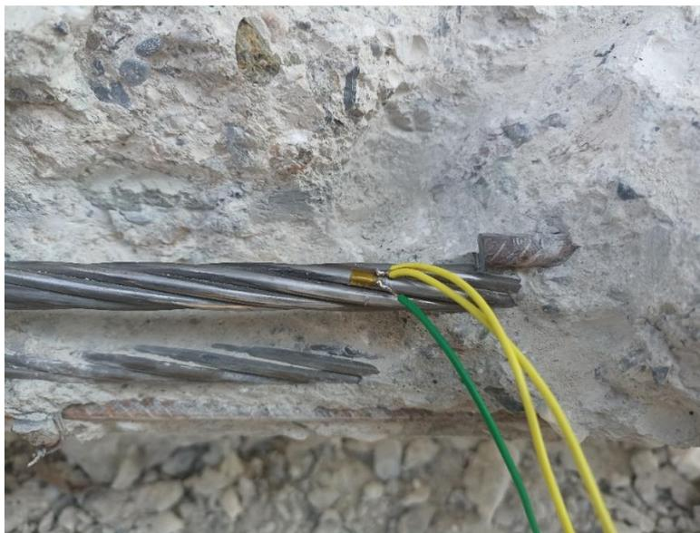
*Figure 29. Strain gauge on the steel strand.*
