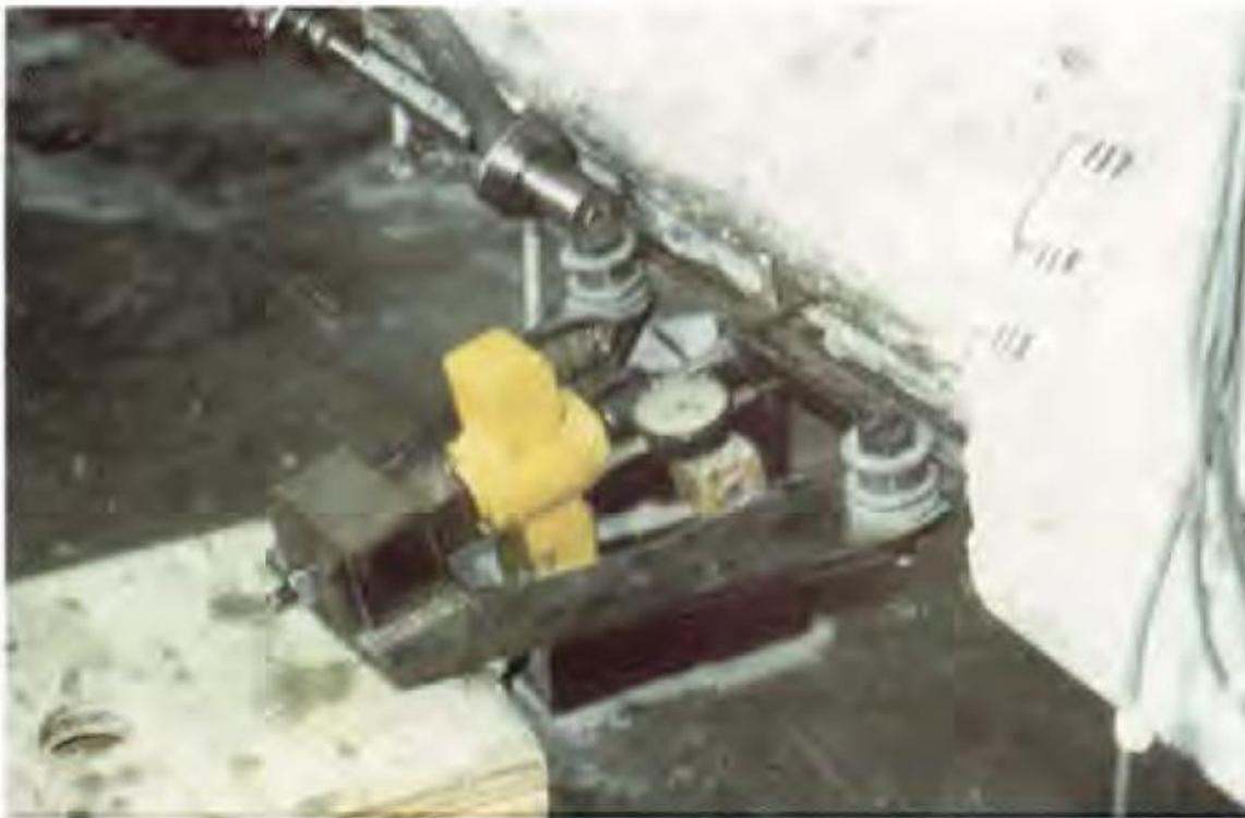
*Figure 16. (Civjan et al., 1998) Prototype during splice test.*
