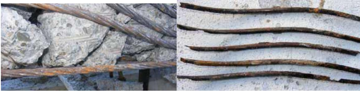
*Figure 7. (a) Broken out strands with uniform corrosion; (b) Individual wires with pitting damage, from (Rogers et al., 2012).*
