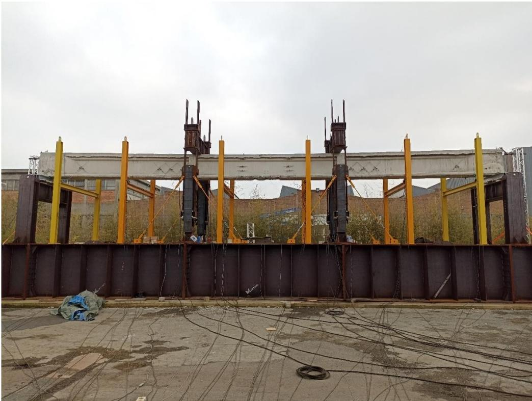
*Figure 24. PC beam on loading frame.*
