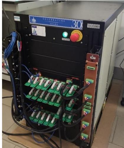
Figure 3. 10 - Arbin battery cycler
