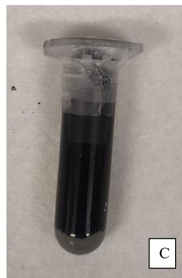
Figure 3. 2 – Micropipette (a), PVdF in NMP solution (b), slurry in the test tube (c)
