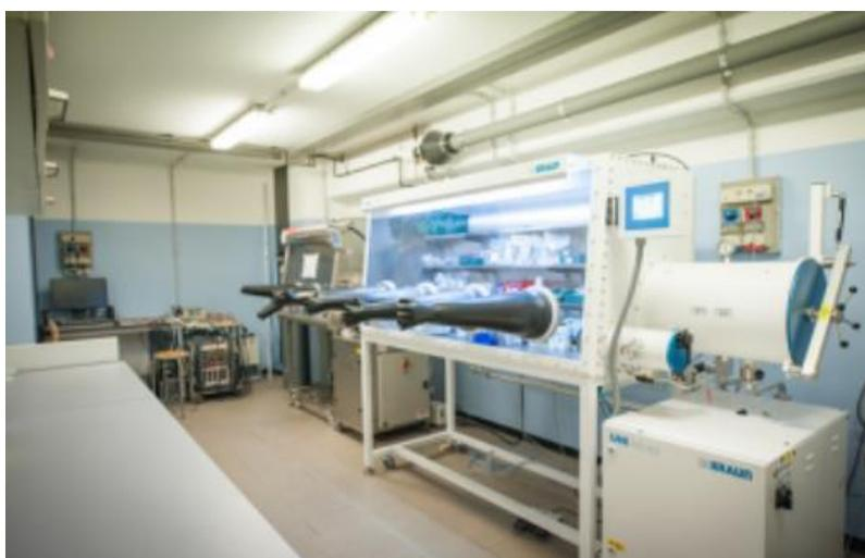
*Figure 3. 7 – Glovebox at DISAT Electrochemistry Lab [35]*
