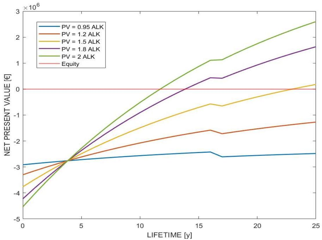
Figure 25. NPV trend for different PV-ALK electrolyzer ratios.
