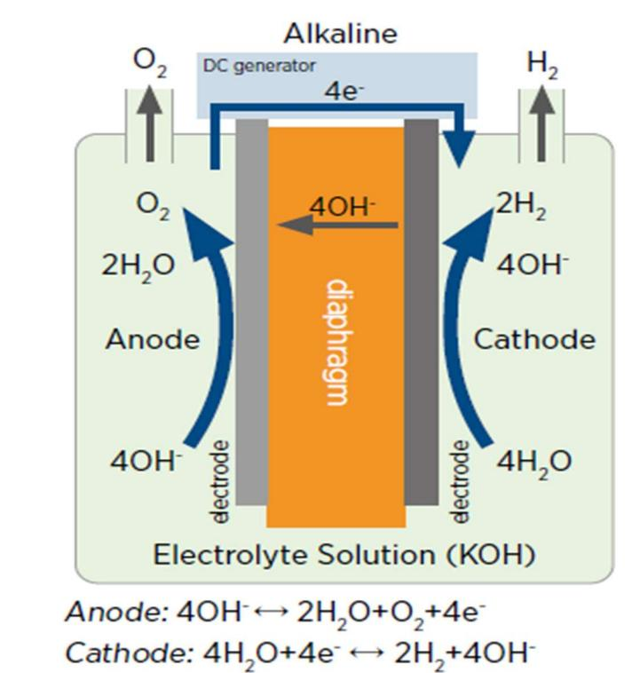
Figure 1. Alkaline electrolytic cell scheme [8].
