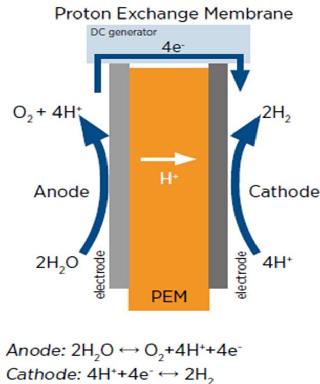
Figure 3. PEM electrolytic cell scheme [8].
