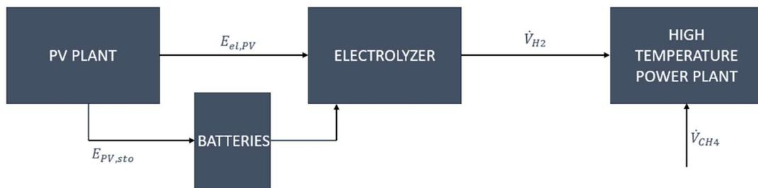
Figure 6. Schematic of the system structure and components.
