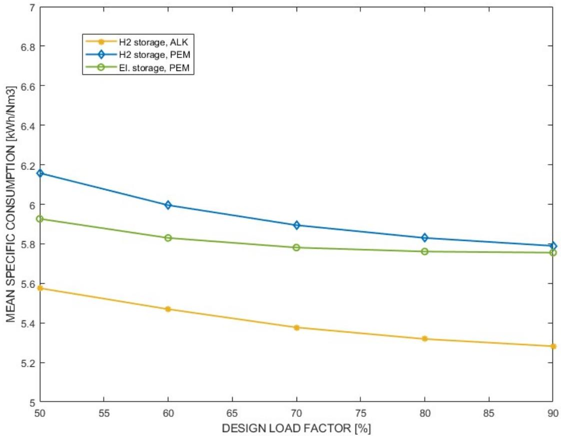
Figure 16. Mean specific consumption by varying the design load factor.
