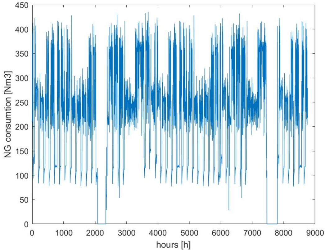
Figure 9. Natural gas consumption hour profile.
