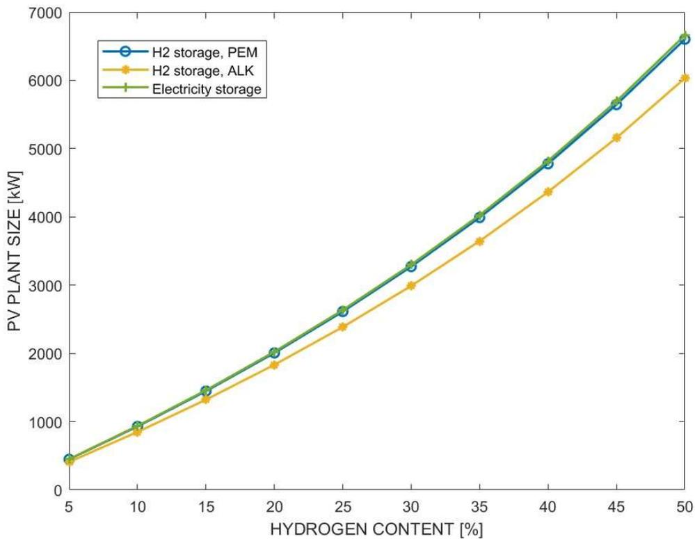
Figure 18. PV plant size as a function of blending.
