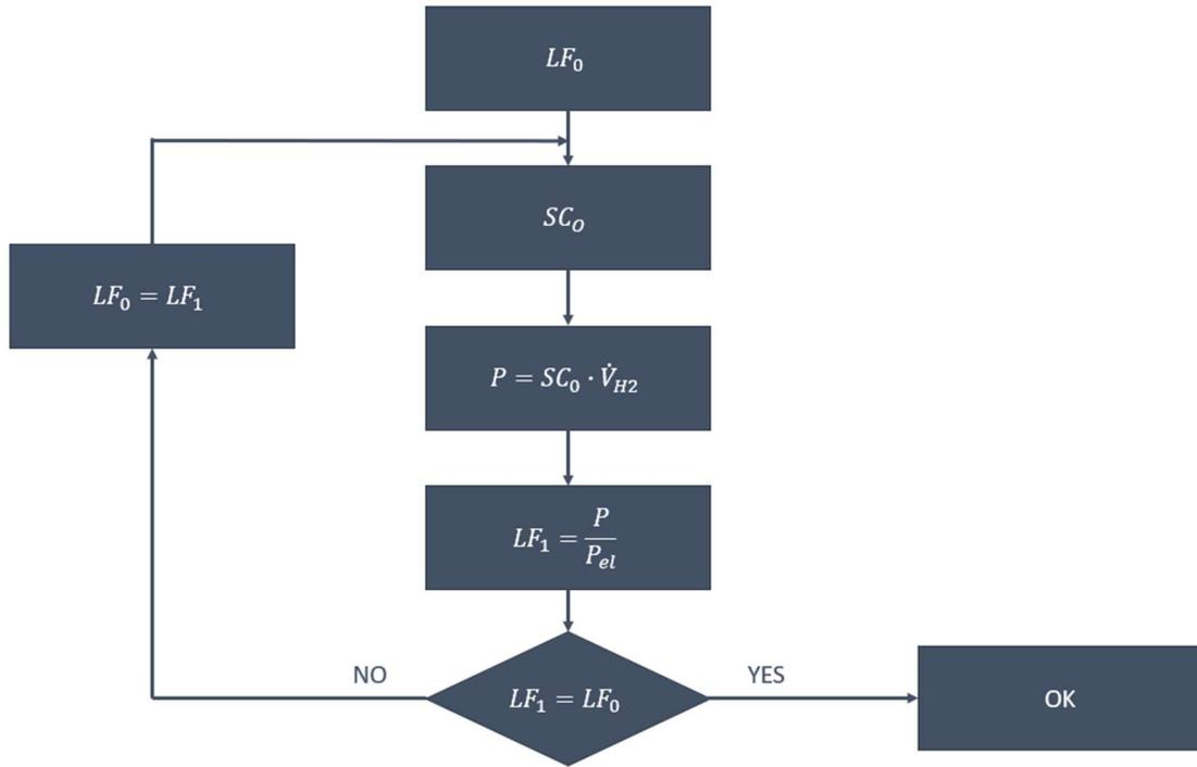
Figure 8. Scheme of the iterative process for the hourly electrolyzer working conditions.
