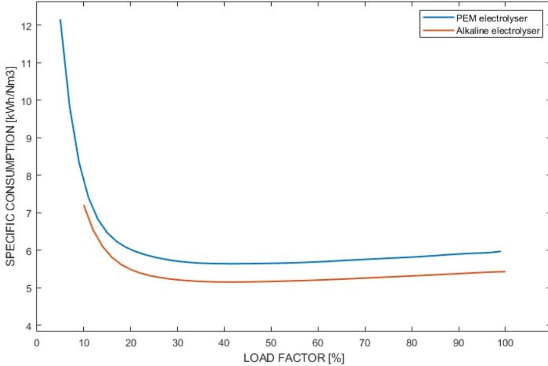
Figure 7. Efficiency curves of PEM and alkaline electrolyzers [13].
