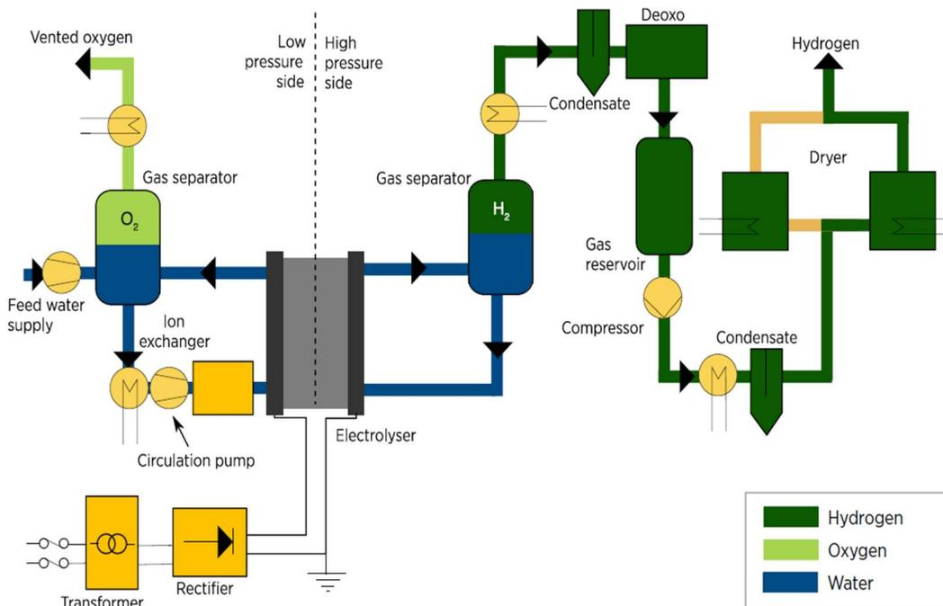
Figure 4. PEM electrolyzer balance of plant [8].
