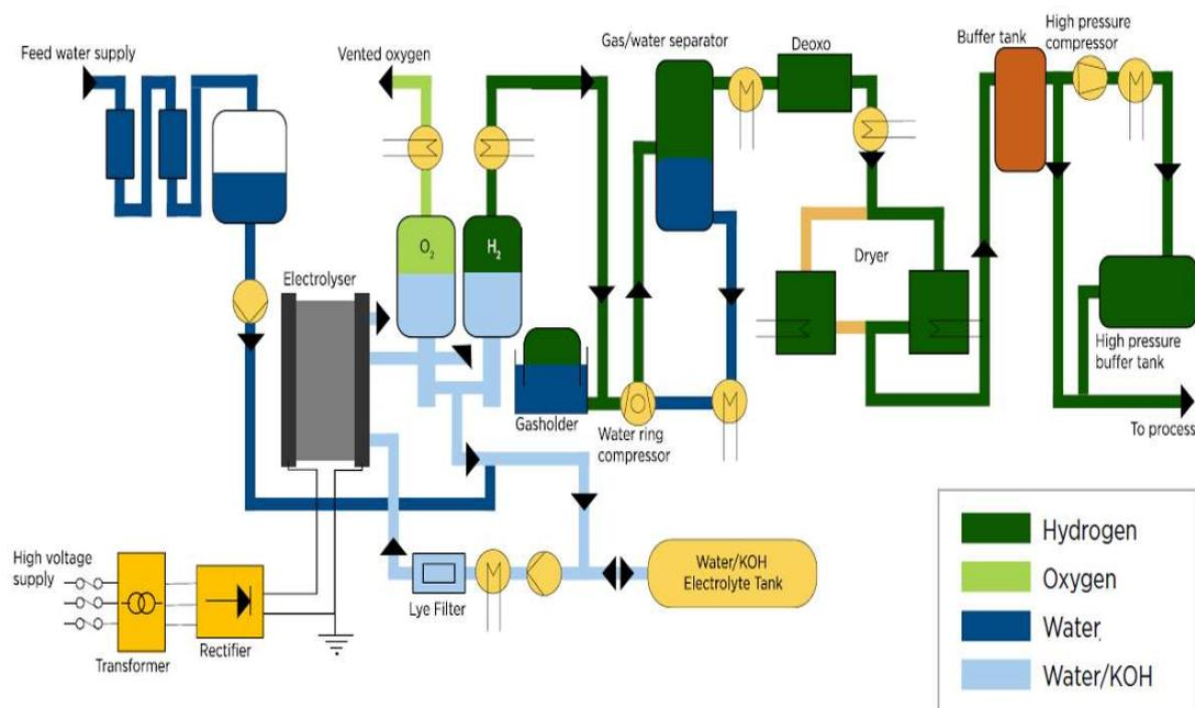
Figure 2. Alkaline electrolyzer balance of plant [8].
