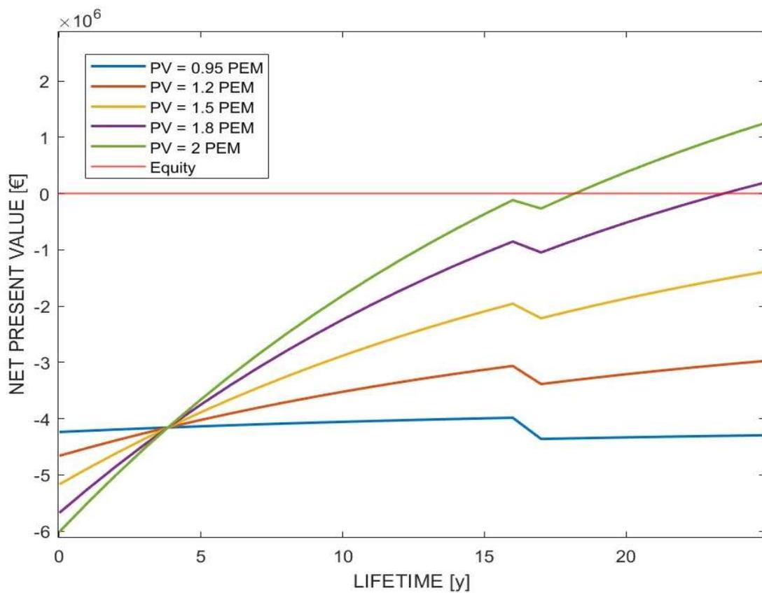
Figure 26. NPV trend for different PV-PEM electrolyzer ratios.
