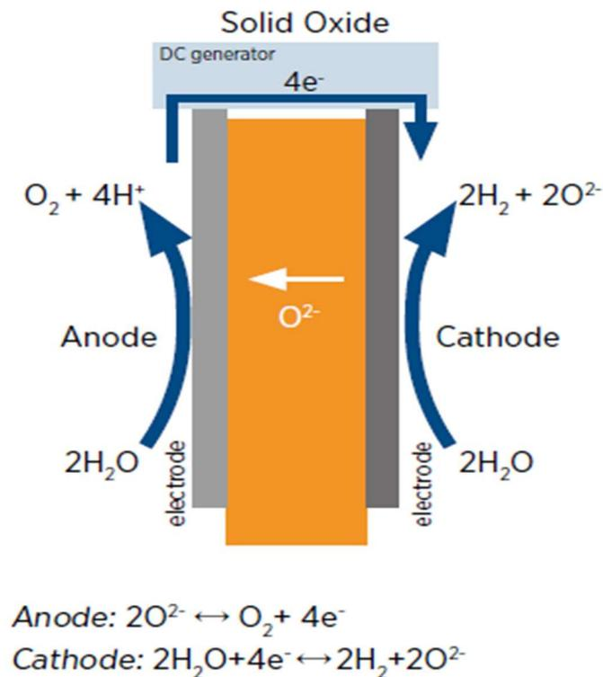
Figure 5. Solid oxide electrolytic cell scheme [8].
