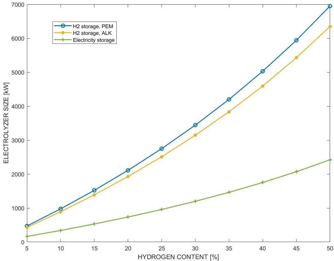
Figure 17. Electrolyzer size as a function of blending.
