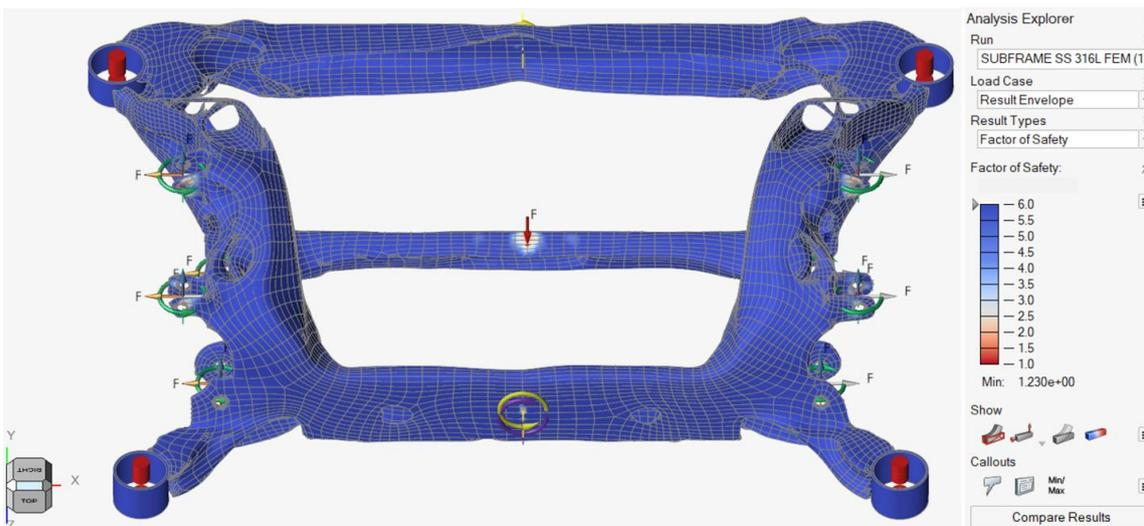
Figure 71. Safety Factor Distribution with SS 316L (Optimized Component)
