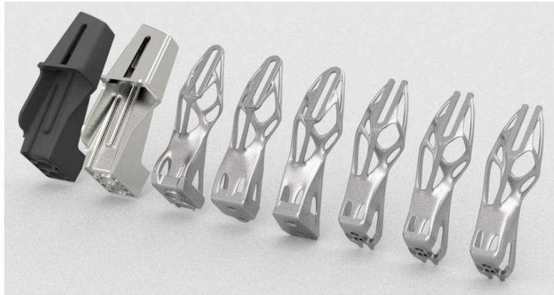
*Figure 20. BMW® i8 Roadster 3D-printed Roof Bracket*
