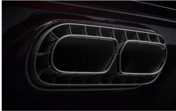
*Figure 24. Bugatti® Chiron Pur Sport 3D-printed Exhaust*
