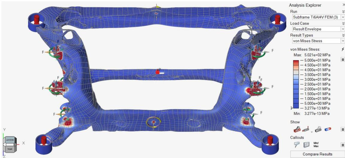
Figure 76. Von Mises Stress Distribution with Ti6Al4V (Top Scale 50 MPa)
