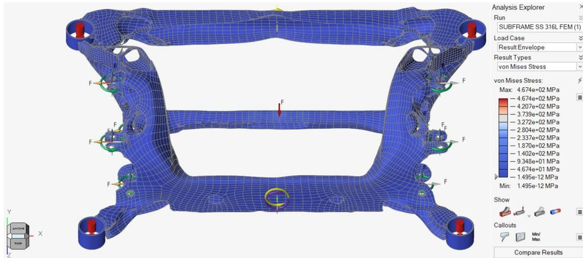
Figure 69. Von Mises Stress Distribution with SS 316L (Optimized Component)
