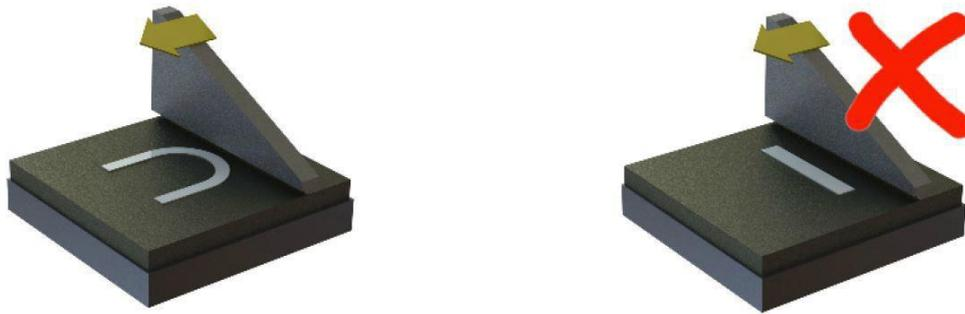
Figure 18. Cross-Section Orientation with respect to Re-Coater Blade Motion
