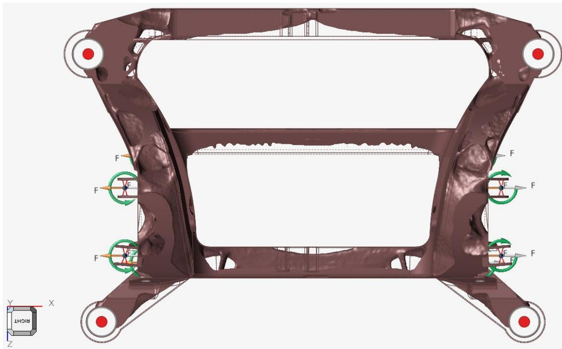
Figure 58. Rear Subframe Topology Optimization with Ti6Al4V (Top View)
