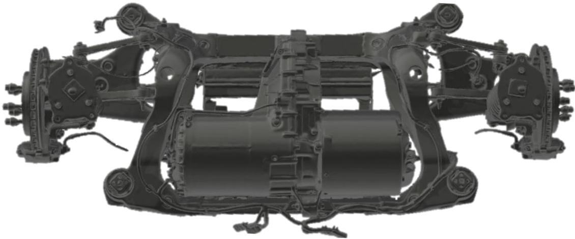
*Figure 31. Rear Suspension Assembly (Top View)*
