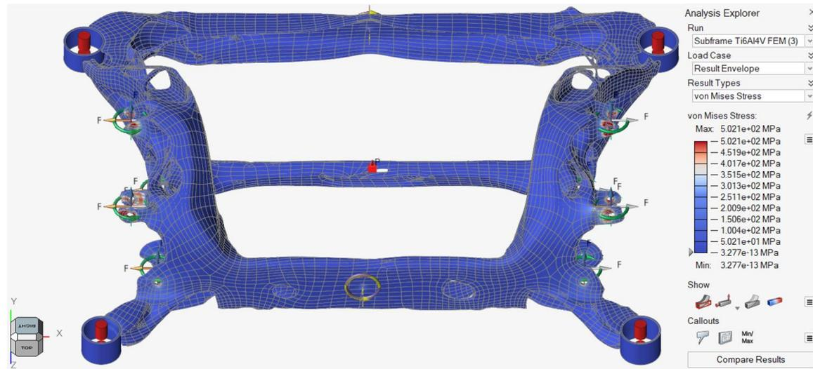
Figure 75. Von Mises Stress Distribution with Ti6Al4V (Optimized Component)
