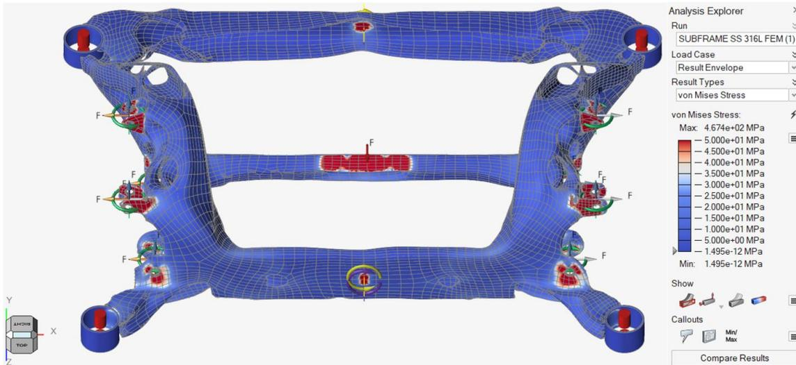
Figure 70. Von Mises Stress Distribution with SS 316L (Top Scale 50 MPa)
