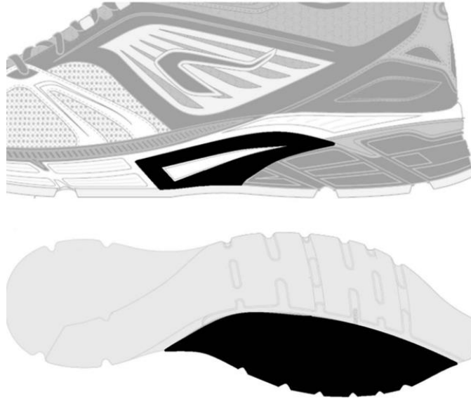
Figure 4.7: Representation of medial/lateral reinforced regions of the midsole of cushioning shoes.
