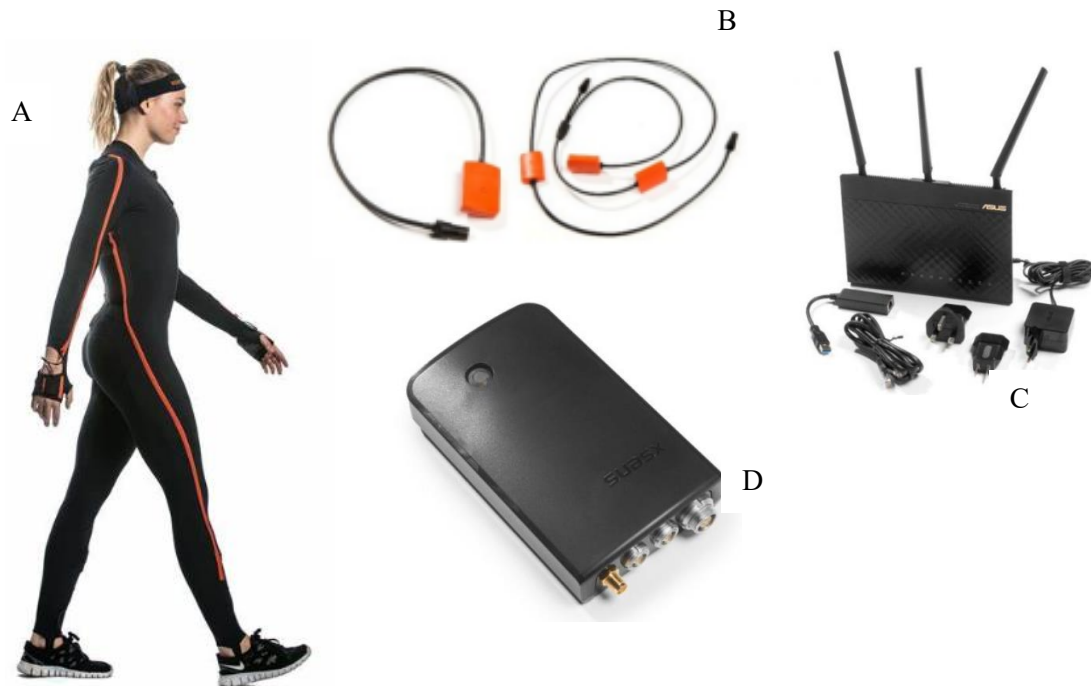
Figure 5.5: Representation of the Xsens 3D Motion Capture System; The suit (A), the MTx's motion sensors (B), the Access Point (C) and the Body Pack (D).
