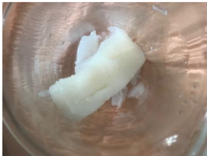
Photo 4.7: Accidental coagulation of SF occurred during a failed attempt of extraction
