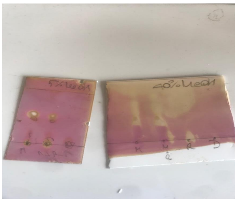
Photo 6.8: Chromatoplates after immersion in \text{KMnO}_4 jar with visible spots
