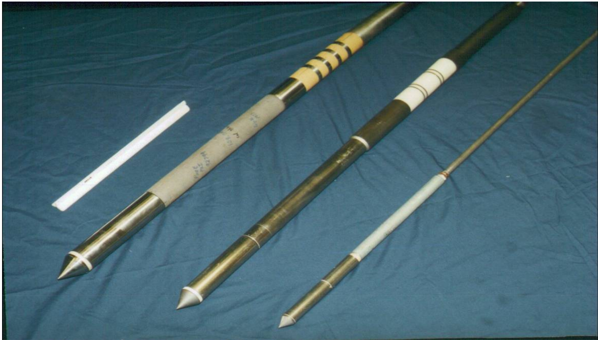
Figure 23 Example of some resistivity cones (courtesy P.Mayne)
