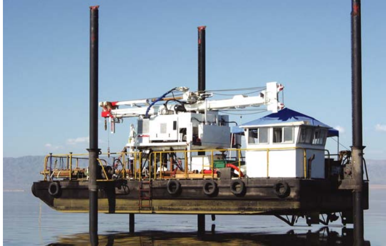
Figure 13 Mid-size jack-up boat
