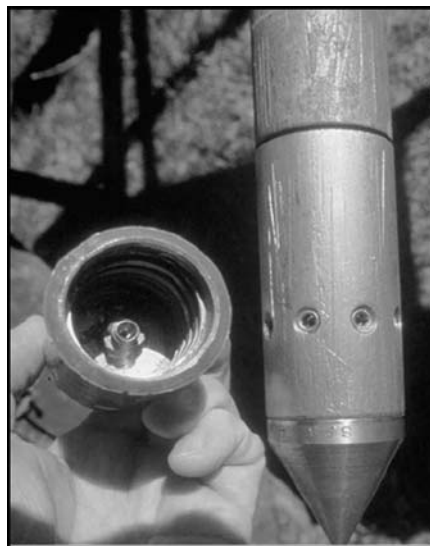
Figure 35 Waterloo profiler probe showing several sampling ports
