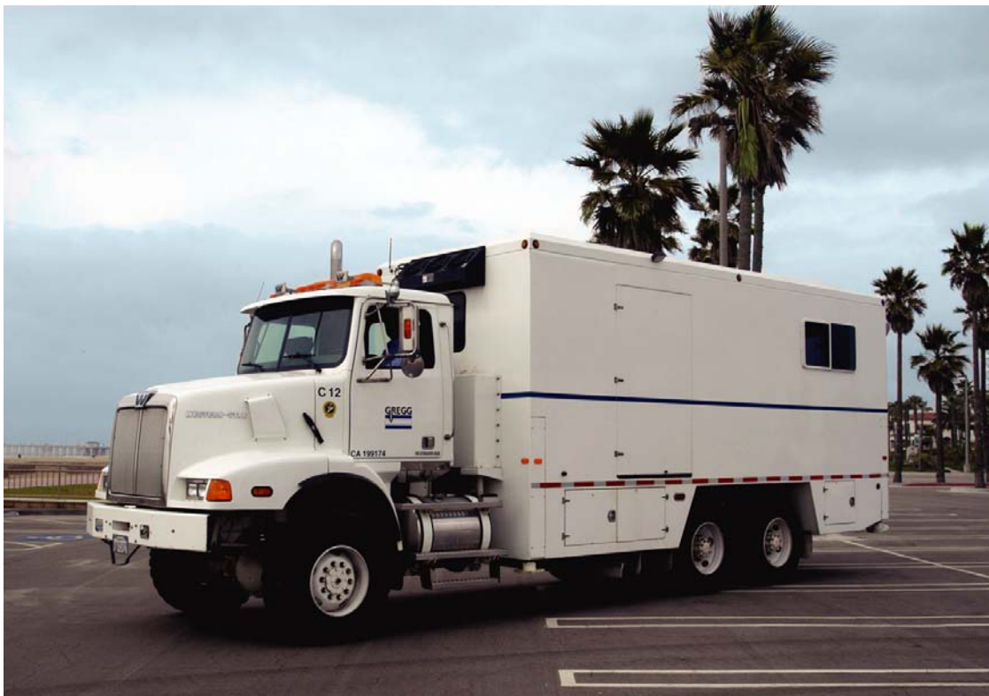
Figure 9 Truck mounted 25 ton CPT unit
