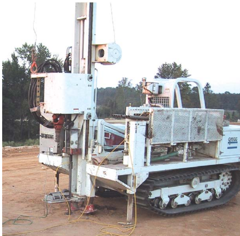
Figure 11 Small anchored drill-rig unit
