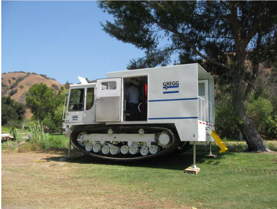
Figure 10 Track mounted 20 ton CPT unit
