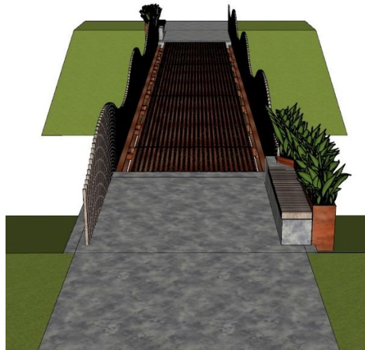
Figure 122. Assembly of perforated Corten steel sheet representation
