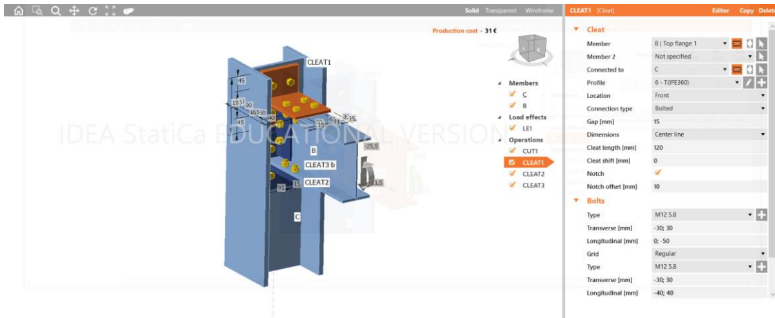
Figure 98. Design of Gantry (HEB200-IPE180) connection (IdeaStatica)
