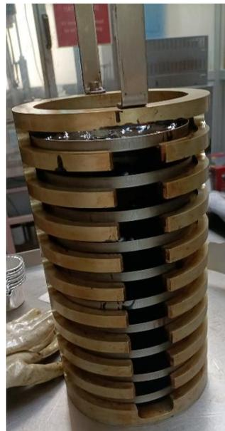
Figure 9 Trays with bitumen
