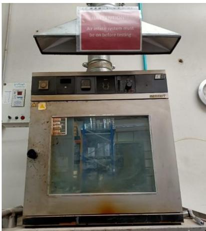
Figure 6 RTFO test oven in the laboratory
