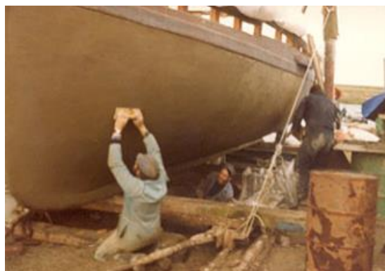
Figure 10 Ferro-cement fishing boat 'La Giuseppa', designed by Nervi, 1967 Image source: ericafirpo.com (left): ferrocement boat name PRISCILLA (right) [10]
