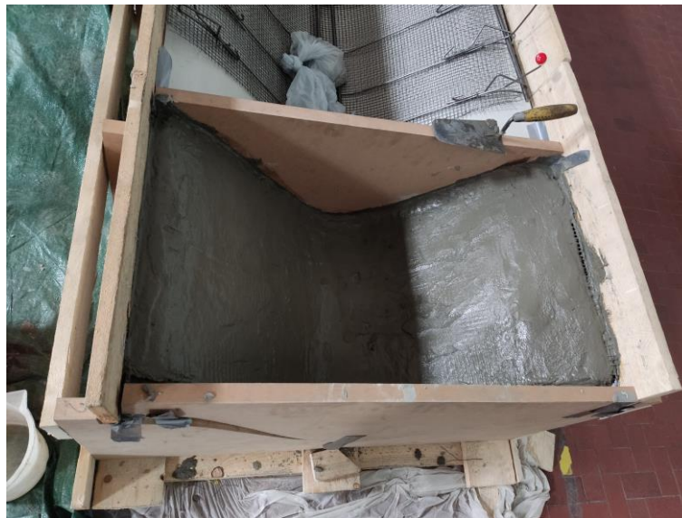
Figure 75 trail casting of the beam
