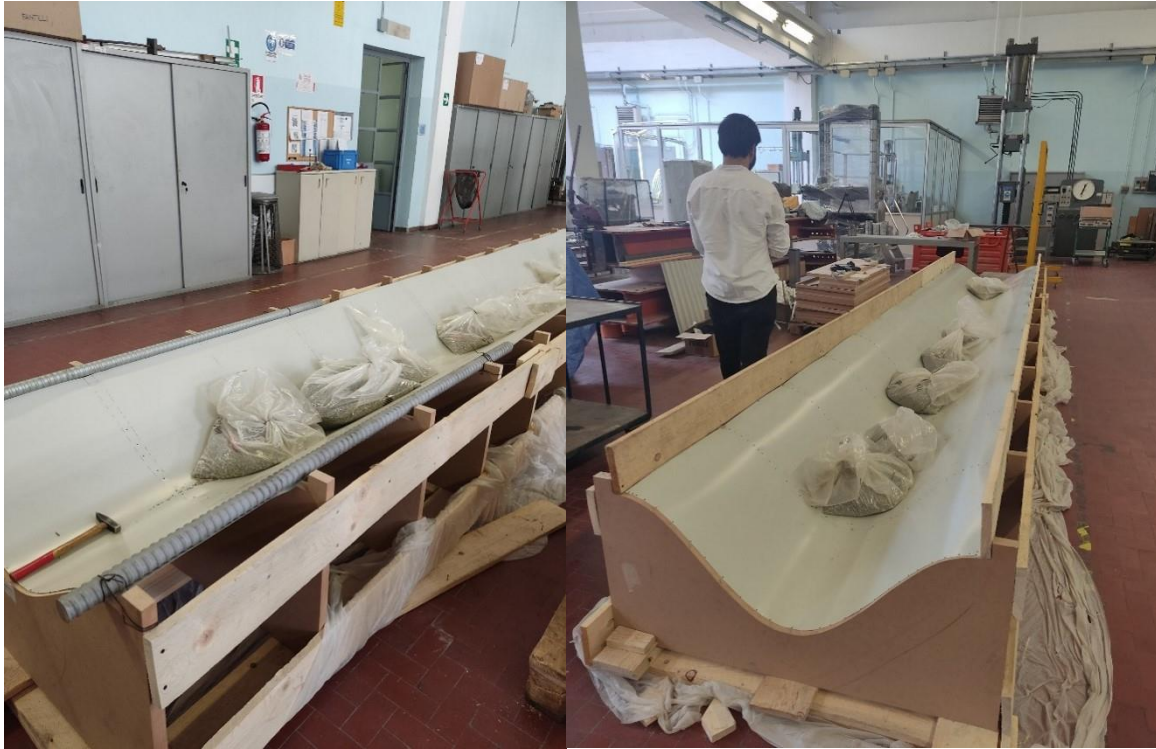
Figure 67 placing of the aluminium sheet
