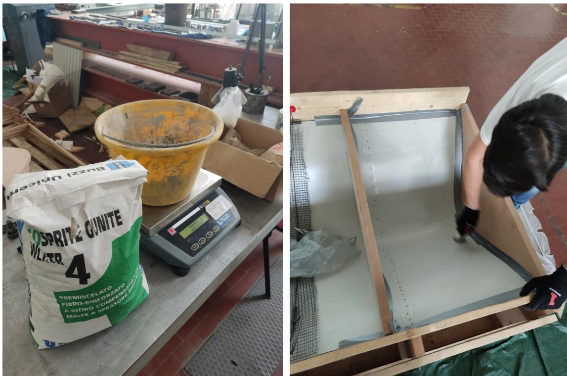
Figure 74 weighing the cements to add the required water and application of the scotch tape.
