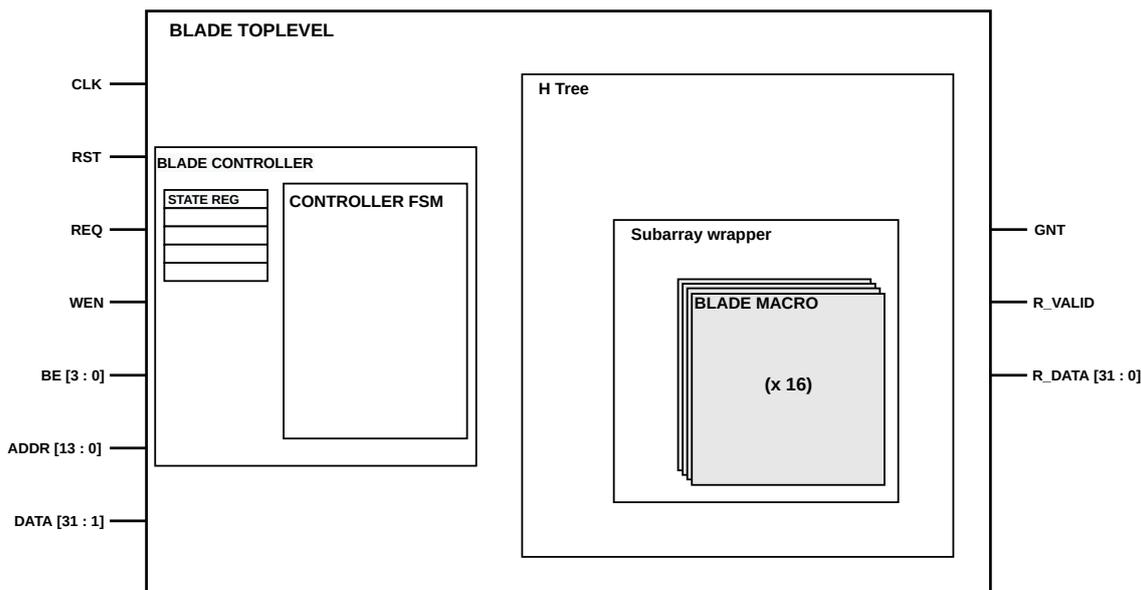
Figure 3.3: New controller general architecture
