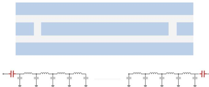
**Figure 2.5:** Realistic representation of a coplanar waveguide resonator; the signal travel along the central conductors of width  $w$ , spaced from the ground plane by a trench of width  $d$ . On the bottom the equivalent circuit representation is shown; the CPW is modeled as an LC distributed transmission line
