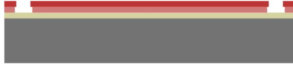
**Figure 5.6:** Ebeam resist development
