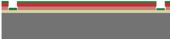
**Figure 5.7:** 5nm of Ti and 55nm of Pt or Pd are evaporated to form the markers
