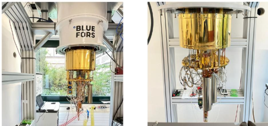
**Figure 6.1:** Blue-fors, dry dilution cryostat.
