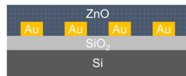
Figure 2. Schematic drawing of the photoresistor devices. Layers and components are not to scale.
