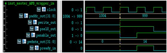
**Figure 3.8:** Write transfer signals toward Interface Memory in customized Trv32p3 microprocessor using AMBA APB system bus.
