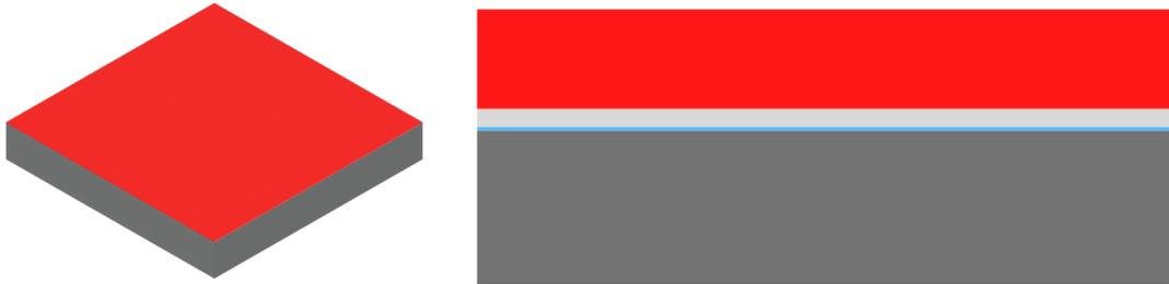
**Figure 3.5:** Photo resist coating of the wafer, over the aluminum layer, after dehydration procedure.
