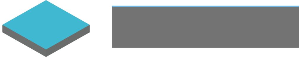
**Figure 3.2:** Silicon wafer after RCA process and  $SiO_2$  deposition
