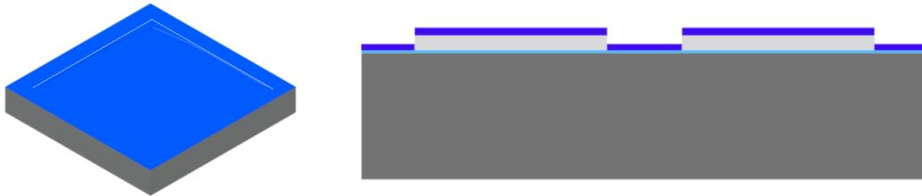
**Figure 3.12:** Silicon dioxide deposition on the front side of the wafer.
