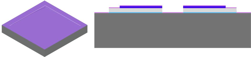
**Figure 3.16:** IrOx deposition on the front side.
