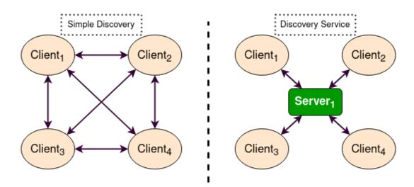
Figure 6.3: Fast DDS Discovery Server
