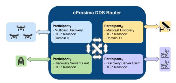
Figure 4.2: eProsima DDS Router local use case
