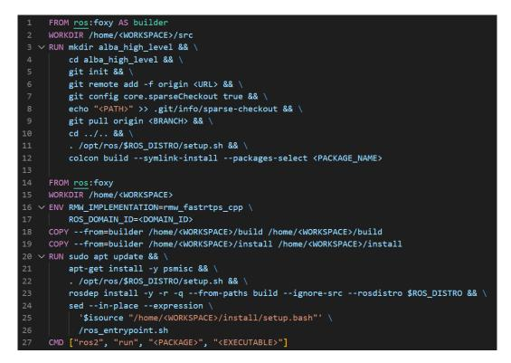
Figure 6.2: Template for containerizing ROS2 nodes
