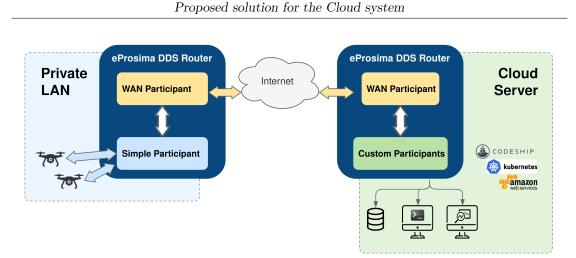
Figure 4.3: WAN communication with the DDS Router
