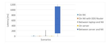
Figure 7.15: Latency distributions with remote communication
