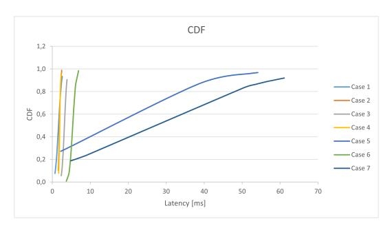
Figure 7.18: Latency required for nodes activation
