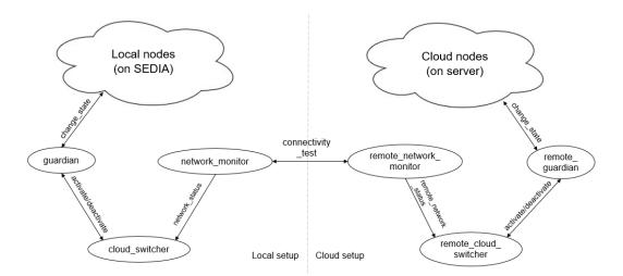
Figure 4.5: Switching mechanism architecture
