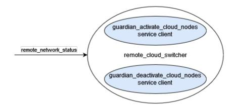
Figure 4.9: The remote\_cloud\_switcher node
