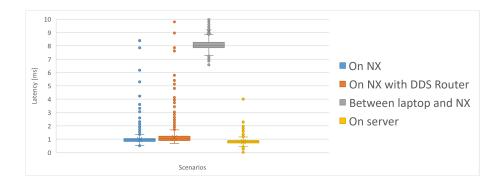
Figure 7.14: Latency distributions without remote communication
