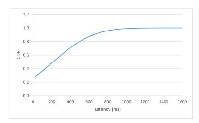
Figure 7.13: Latency between NX and server with enhanced performance
