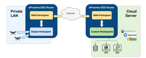
Figure 6.4: WAN communication with the DDS Router
