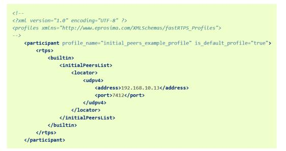
Figure 4.1: XML configuration file for an Initial Peers List
