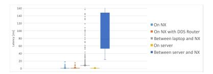
Figure 7.16: Latency distributions with remote communication with enhanced performances
