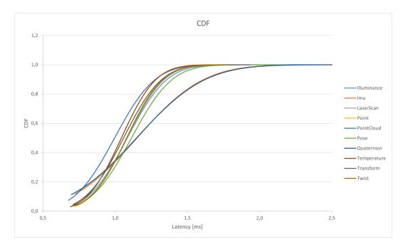
Figure 7.4: Latency on NX with DDS Router
