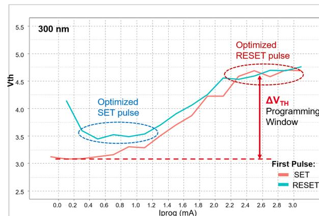
Figure 3.12: Same graph as in figure 3.11, here the optimized current values for SET and RESET pulses are highlighted; the threshold voltage window  $\Delta V_{TH}$  is the difference between full SET and RESET  $V_{TH}$ .
