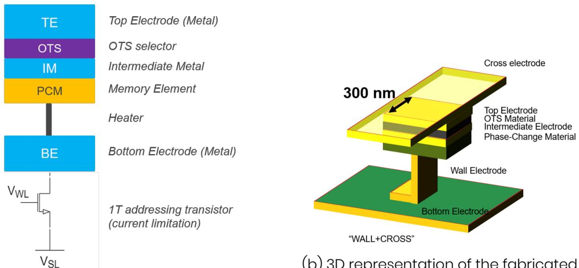
(a) Circuit scheme of the selector and memory stack, OTS is sandwiched between the Top Electrode (BL) and an intermediate electrode.
