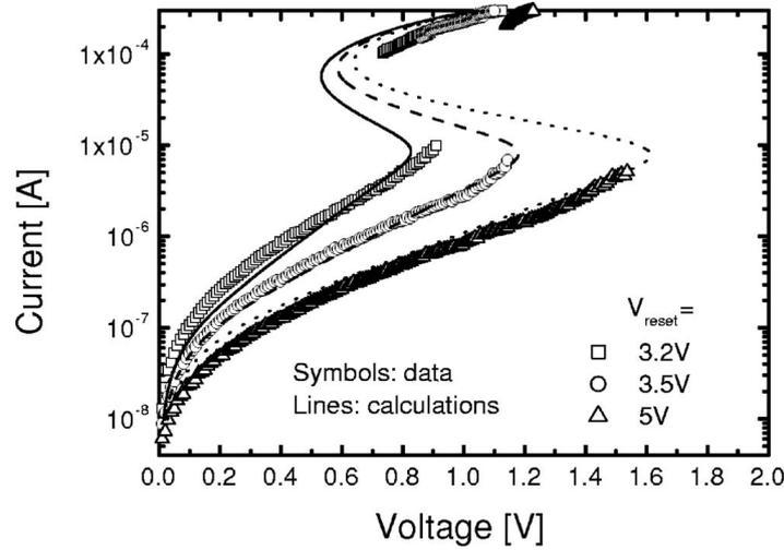
Figure 2.17: Experimental (shapes) and calculated (lines) data for three different PCM programming pulses ( $V_{reset}$ ), each one corresponding to an increased volume of the amorphous phase. The sub and above threshold have good agreement while in the threshold region the model does not fit the experimental data [14].
