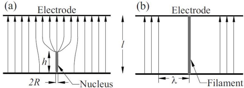
Figure 2.18: Field Screening effect that happens for (a) a conductive nucleus (supposedly cylindrical) of height  $h$  and radius  $R$ . The electric field concentrates at the tip and is weakened around it; the filament grows until it shorts the electrodes (b).
