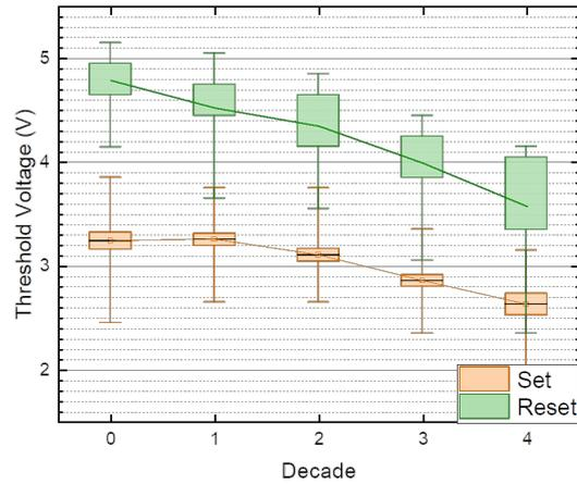
Figure 3.15:  $V_{th}$  for SET and RESET state reported as a function of the cycling decade. The solid box represents the standard error while the whiskers show the outlier elements.
