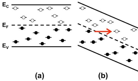
Figure 2.15: Low-field (a) and High-field (b) electrons energy distribution scheme. With Low or No field applied all the electrons fill trap states below the fermi energy; when the applied field increases, TE and tunneling are favored and electrons fill higher energy traps [14].
