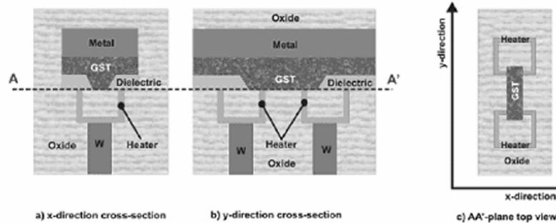
Figure 2.8:  $\mu$ Trench Cell shares a similar working principle to the Wall-Heater structure but uses a thin trench filled with metal to form the heater and allows for multiple close cells integration [13].
