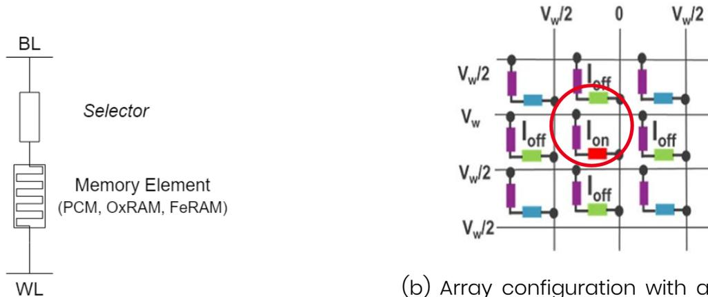
(a) Circuit scheme of a selector and memory stack, bias is applied across Bit-Line (BL) and Word-Line (WL)
