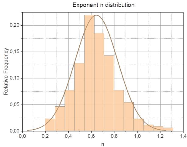
Figure 3.7: Exponent  $n$  distribution, the current is proportional to the exponent of the voltage at the  $n$ th power. Within experimental error, the coefficient appears close to 0.5 implying the dominant contribution of Poole-Frenkel conduction type.
