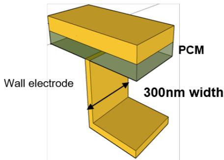
(a) 3D model of the tested PCM, the wall electrode shaped like an "L" is placed at the bottom of the memory layer.
