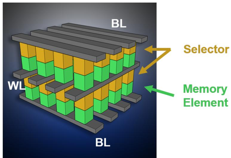
Figure 2.22: Crossbar architecture scheme, here reported for two layers. WL is in the middle perpendicular to the BL above and below, selectors are depicted in mustard while the memory element is in green.
