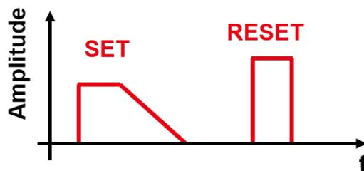
Figure 3.2: SET and RESET pulse scheme, here *Amplitude* is the current during the pulse, the SET pulse has a long fall time while the RESET pulse has a short fall time to ensure the amorphization of the melted region.
