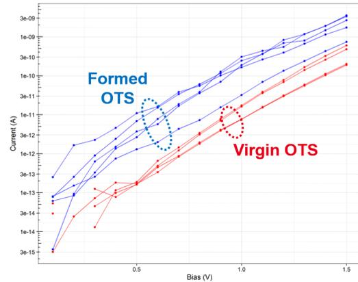
(b) Subthreshold characteristic comparison. In Red are the curves for five virgin (as deposited) devices, and in blue are reported the same devices after the FF step.
