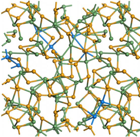
Figure 2.19: Simulation of 72 atoms random network. In blue are highlighted the new Ge-Ge bonds formed with switching [21].
