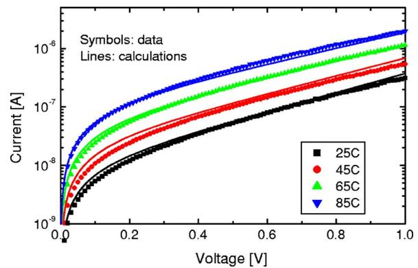
Figure 2.14: Measured and calculated  $I-V$  curve for increasing temperature; is possible to appreciate the linear regime for voltages lower than  $0.2V$  followed by the exponential regime up to  $1V$ . Adapted from [14].
