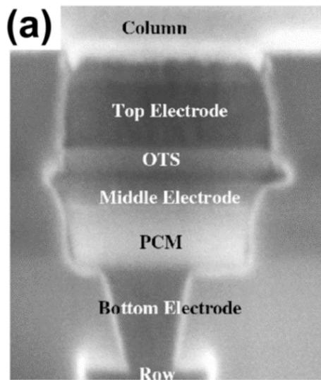
(a) Memory device from [24], the heater corresponds to the Bottom Electrode.
