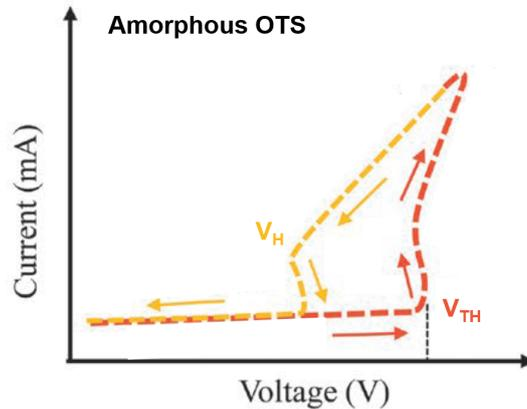
Figure 2.12: General switching characteristic of an OTS material, at  $V_{TH}$  it starts conducting with a voltage snap-back; the device remains in the ON state until the voltage is lowered below  $V_{hold}$ .
