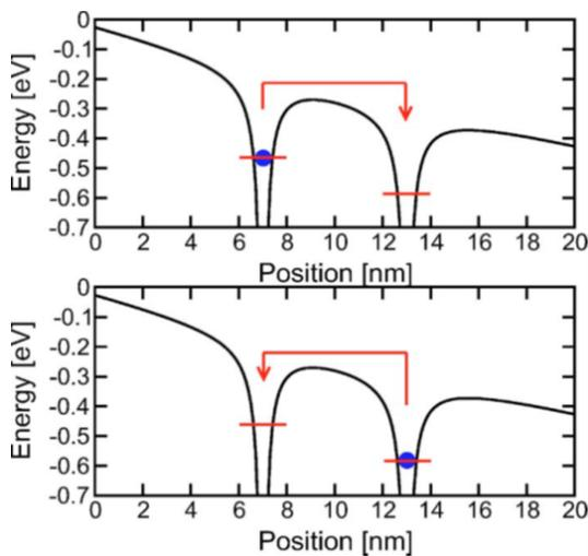
Figure 2.13: Poole-Frenkel model for conduction, the electrons are trapped in potential wells due to the defective nature of the amorphous phase. Electrons may tunnel and move from one trapped state to the other due to thermal emission, when an Electric field is applied, current in one direction is favored [14].
