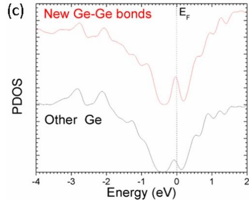
Figure 2.20: Partial Density of States of the newly formed Ge-Ge bonds close to  $E_F$ , compared to neighboring Ge sites in the excited state [21].
