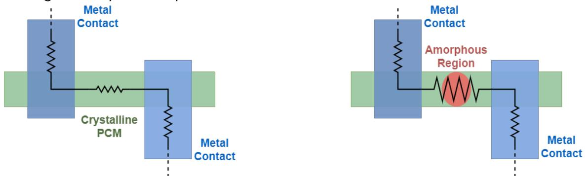
(a) PCM in the crystalline state has low resistivity (here pictorially shown as a small resistor).
