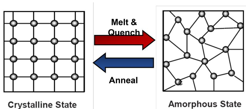
Figure 2.2: Pictorial representation of the stable ordered crystalline phase (on the left) and the metastable disordered amorphous phase (on the right). When the material is melted and quenched, it amorphizes; on the contrary, it will crystallize after an annealing step.
