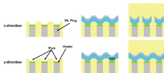
Figure 2.7: Pore Structure: due to the narrow pore filled with chalcogenide material, the high current density will heat the region in a similar fashion to the Wall-Heater structure [11].
