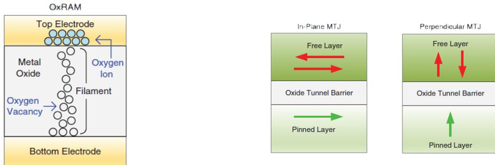
(a) RRAM based on Oxygen vacancies, when programmed a conductive filament is formed while once RESET the filament is destroyed and the resistance of the cell increases.
