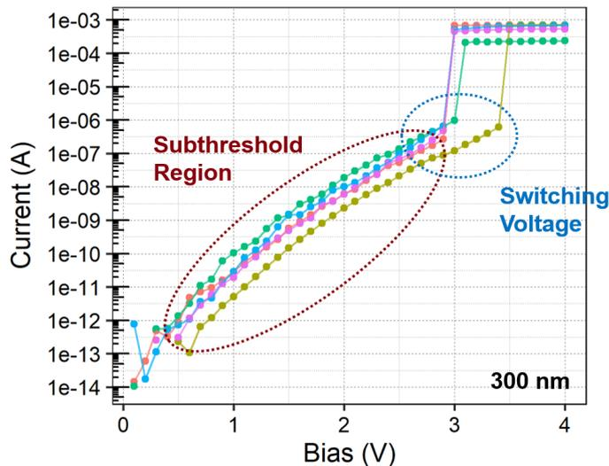
Figure 3.5:  $I/V$  Characteristic of five devices, subthreshold and threshold region are circled.
