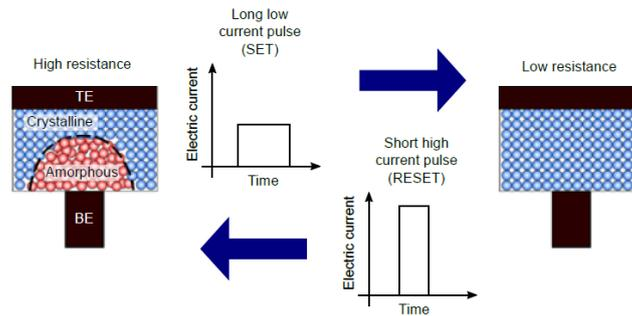
Figure 2.5: SET and RESET pulse of a PCM vary in amplitude and duration to reach either crystallization or melt-quenching. High-intensity pulse melts a portion of the material while a long but lower pulse may achieve crystallization of the layer. From [12]
