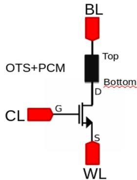
Figure 3.16: Circuit scheme of a single device in the array structure, that is identical to the ones described in section 3.2
