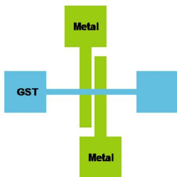
Figure 2.6: Bridge structure is made by a layer of chalcogenide material deposited on top of two parallel metal electrodes. Since the structure is symmetric the hot spot is located close to the center of the bridge [11].
