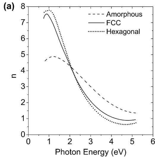
Figure 2.3: GST-225 refractive index variation as a function of the photon energy, the long dash line is the amorphous phase while the solid line is the stable crystalline FCC phase; the short dash line is the metastable hexagonal crystalline phase.
