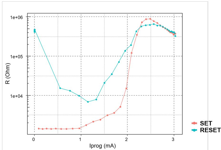
Figure 3.3: Resistance of the PCM after an applied programming pulse of intensity  $I_{prog}$ .
