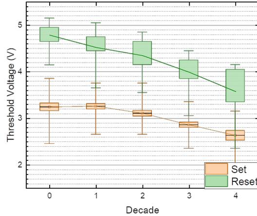
Figure 3.15:  $V_{th}$  for SET and RESET state reported as a function of the cycling decade. The solid box represents the standard error while the whiskers show the outlier elements.
