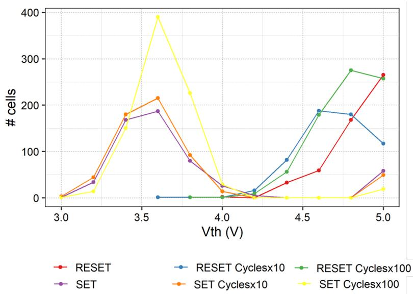
Figure 3.18: Threshold voltage distribution for a 1kbit array of devices, the two distributions show SET and RESET state  $V_{th}$  for a few cycles.
