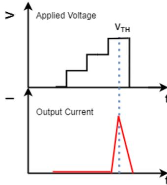
Figure 3.9: Reading staircase step: a voltage staircase is applied to the device and the current is read, when a spike of current is detected it means that the device has switched. After switching the voltage value is stored and the sequence is stopped to avoid damaging the cell with high currents for a long time.
