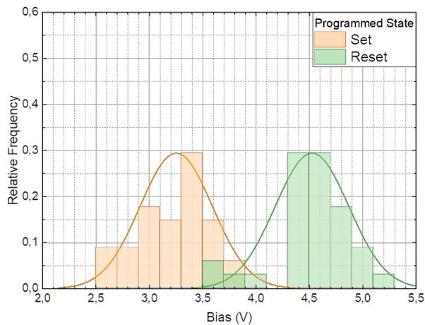
Figure 3.14: Threshold voltage distribution for the two possible states. Distribution appears quite broad indicating a large variability in the process. The overlapping tails correspond to an increase of the BER in the memory.
