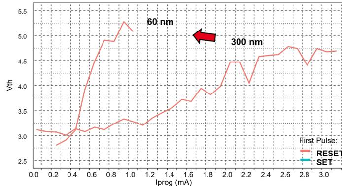
Figure 3.13: Effect of size on the threshold voltage. The adopted protocol is the same, the data for  $300nm$  devices is reported alongside the curve for a  $60nm$  wall width device.
