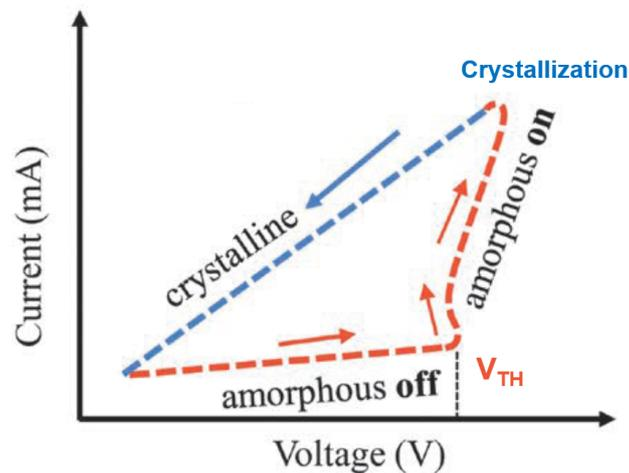
Figure 2.9: OTS switching characteristic [9]. When the amorphous layer switches (red curve), a high current passes, if this current is properly controlled then is possible to exploit Joule heating to crystallize the cell (blue curve).
