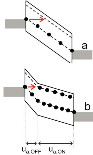
Figure 2.16: Close to the threshold voltage, the electric field is high but the current in the device is still low (a). Upon switching, electrons are accelerated and after a distance  $u_{a,OFF}$ , they reach the conduction band. The mobility in the conduction band is much greater and the voltage drop on  $u_{a,ON}$  is much lower [14].
