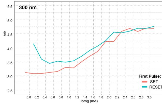
Figure 3.11: Protocol results for the DUT, the curve of the SET protocol in red while the RESET one in blue. The curve is obtained by averaging the characteristic of about 40 devices.
