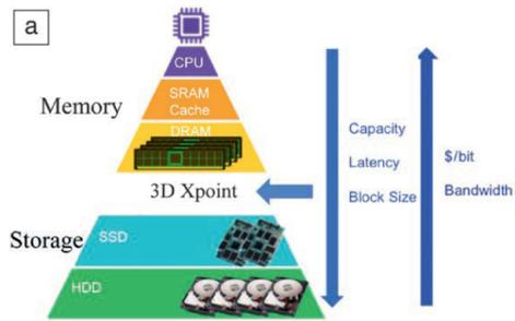
(b) Memory hierarchy in modern computer based on Harvard architecture: Each memory level transfers data from the underlying one in the pyramid. Closer to the CPU, access time is faster but the size is limited; Storage Class Memory offers larger densities and non-volatility, aiming to fill the gap between Main and Mass Memory.
