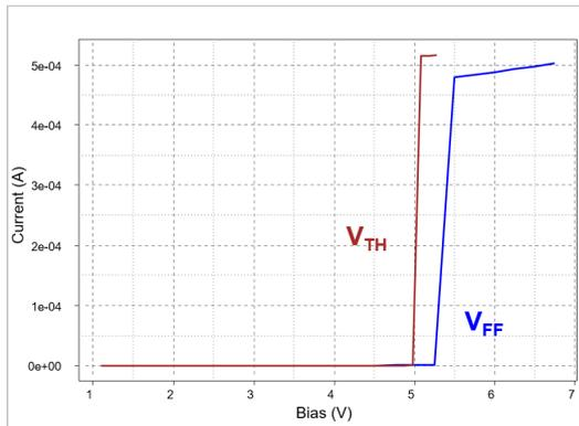
(a) I/V characteristic that shows the threshold voltage during First Fire step and the highest threshold voltage during RESET for the same device.
