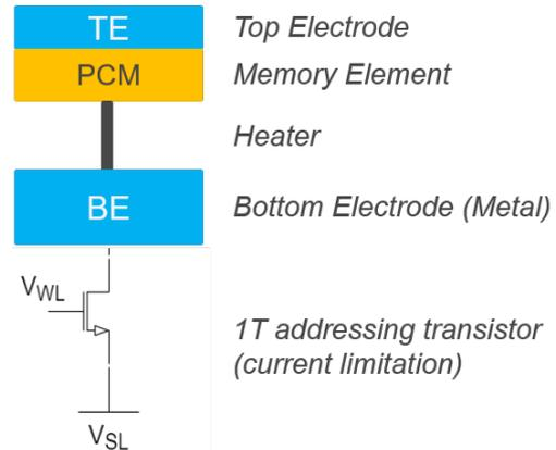
(b) Pictorial Circuit representation of device (a), the series current limiting transistor is shown with its circuitual symbol.
