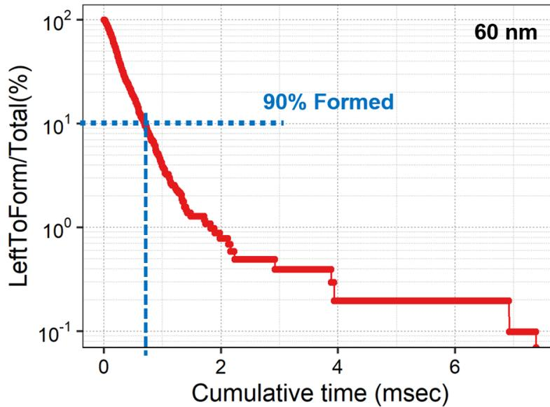
Figure 3.17: Percentage of devices that are yet to be formed over the cumulative time of the forming pulse. After many repeated pulses, each device may stochastically fire: after about  $1ms$  more than 90% of the array has successfully fired.
