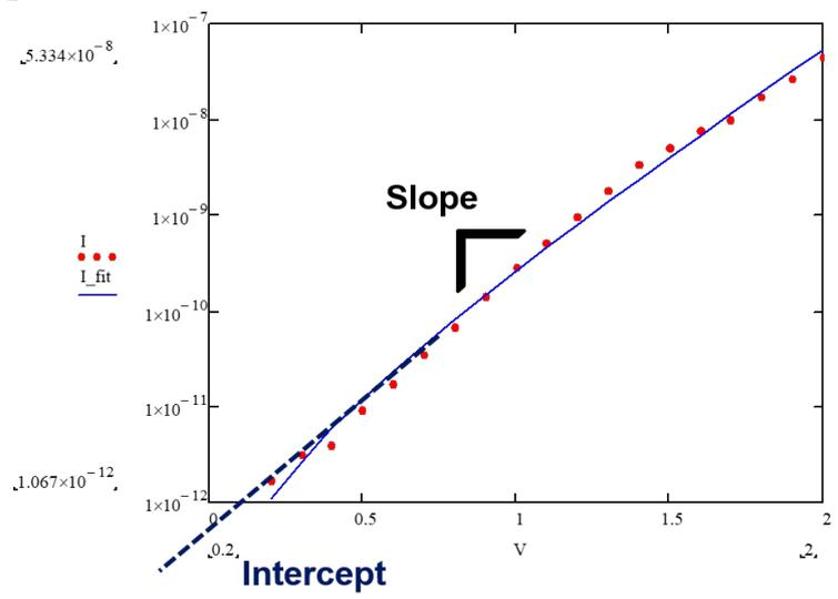
Figure 3.6: Experimental points (red) and fitted line (blue) of the subthreshold  $I/V$  characteristic for a single device. This model extrapolation has been performed multiple times for over 40 devices to acquire sufficient data on the slope and intercept of the lines.
