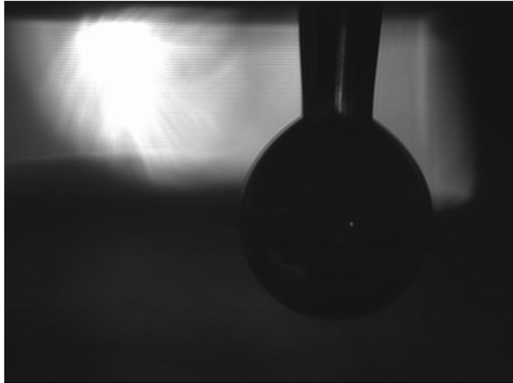
Fig. 2.24 Positive back-pressure result: a big droplet ejected from the nozzle, snapshot taken by the lateral camera.
