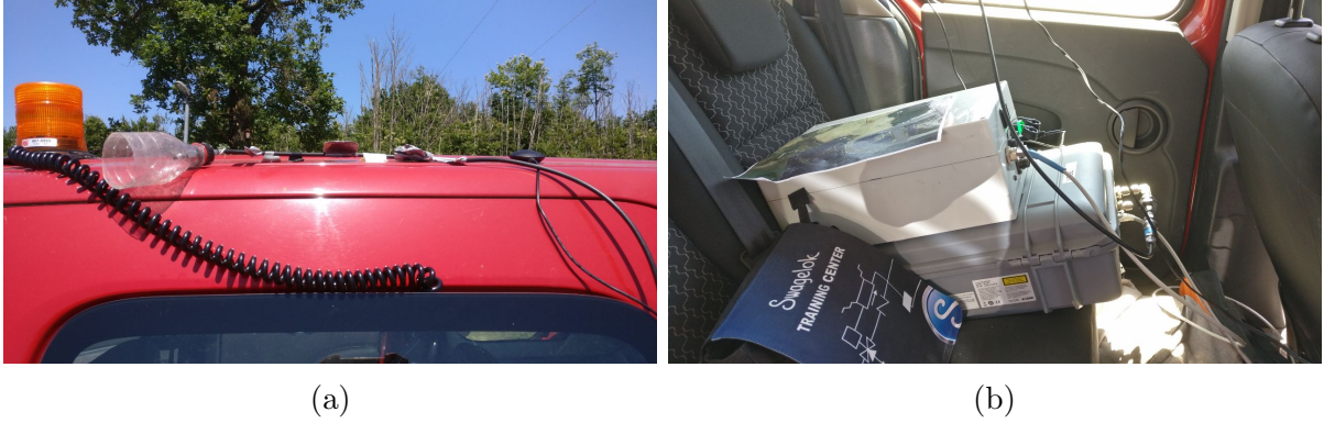
Figure B.2: B.2a: the air inlet (half bottle) is kept above the car for the whole measurement. B.2b: The inlet is connected to a LI-COR analyzer and to a GPS logger inside the car.
