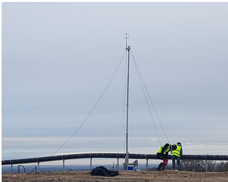
Figure B.1: 3D Sonic Anemometer installed in the center of the landfill.
