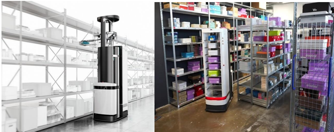
Fig24. Toru robot is picking and storing items from rack
