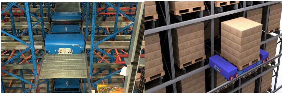
Fig 36. Esmart Shuttle used in AVS/RS is loading/unloading a pallet.
